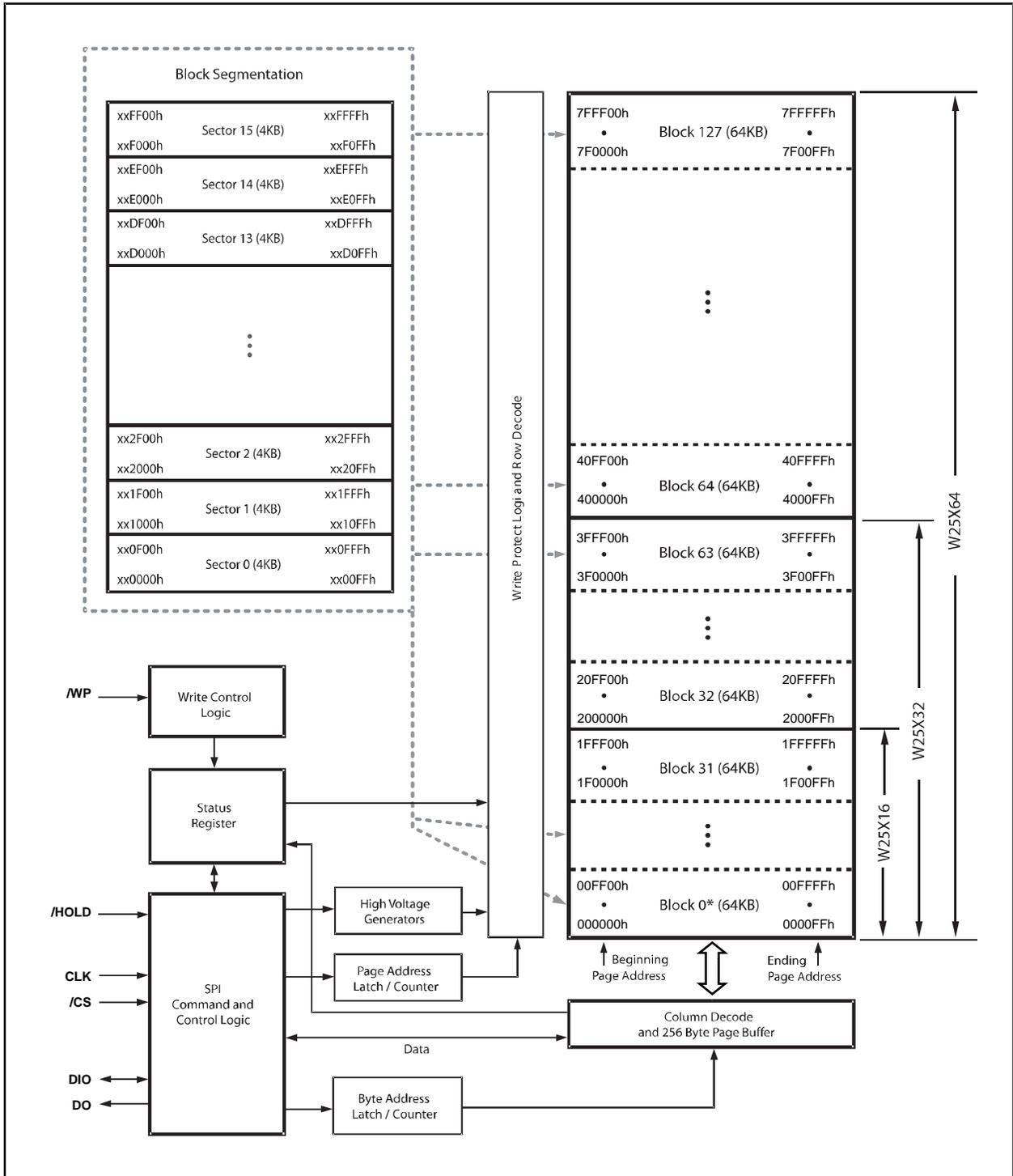
Figure 2. W25X16, W25X32 and W25X64 Block Diagram
