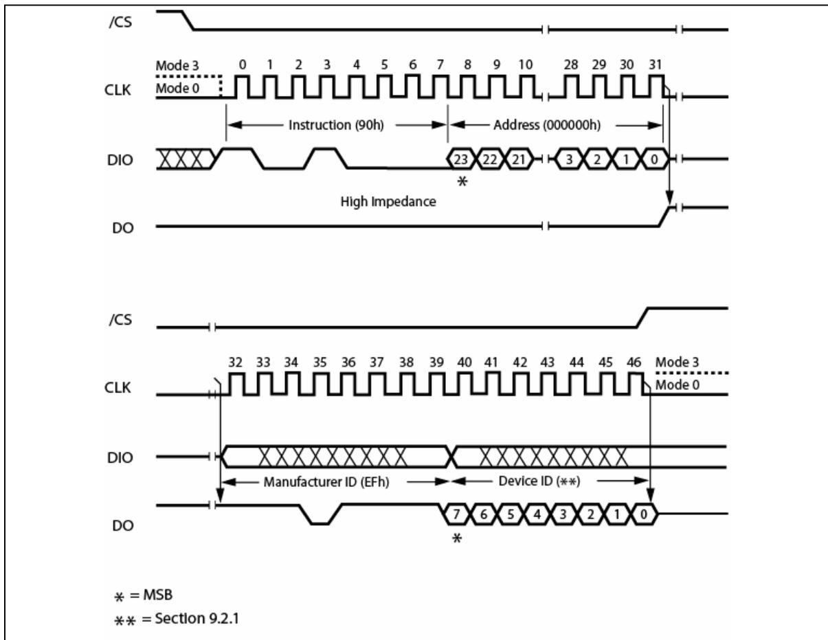
Figure 18. Read Manufacturer / Device ID Diagram
