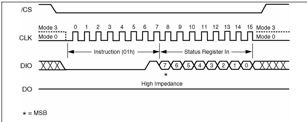
Figure 7. Write Status Register Instruction Sequence Diagram
