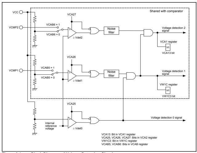
Figure 6.1 Block Diagram of Voltage Detection Circuit
