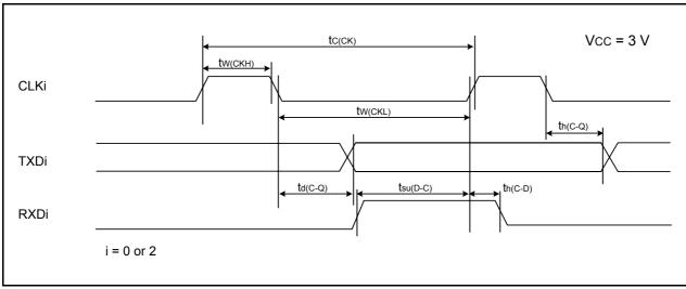
Figure 22.9 Serial Interface Timing Diagram when Vcc = 3 V
