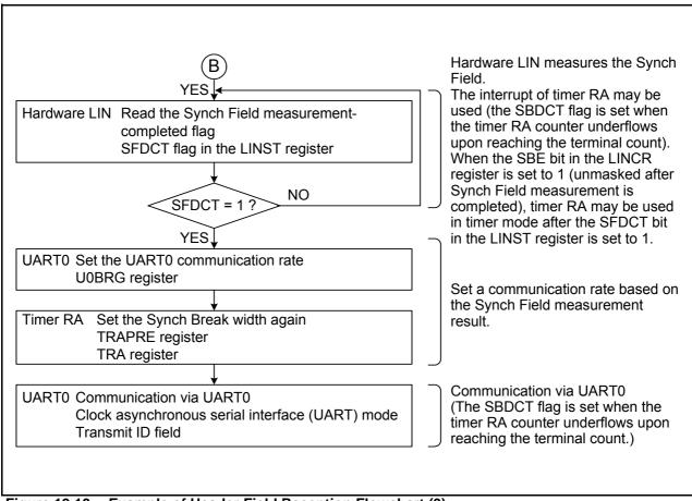
Figure 19.10 Example of Header Field Reception Flowchart (3)
