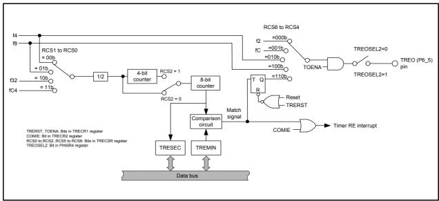
Figure 17.37 Block Diagram of Output Compare Mode
