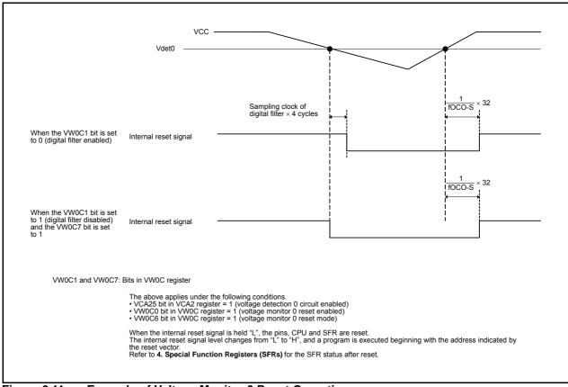
Figure 6.11 Example of Voltage Monitor 0 Reset Operation
