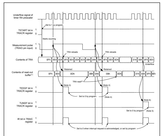
Conditions: The period from one rising edge to the next rising edge of the measured pulse is measured (TEDGSEL = 0) with the default value of the TRA register as 0Fh.
