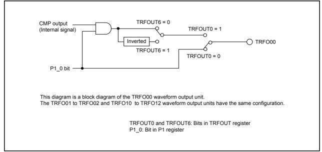
**Figure 17.47 Block Diagram of CMP Waveform Output Unit**
