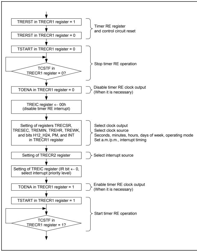
Figure 17.44 Setting Example in Real-Time Clock Mode
