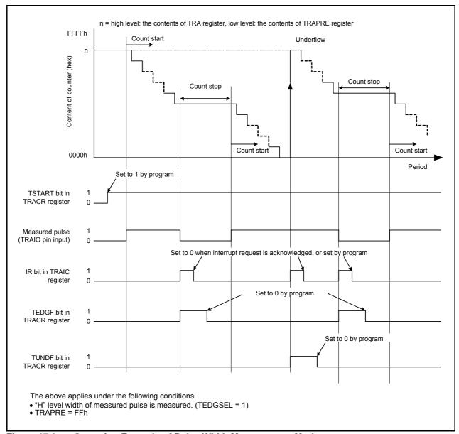
Figure 17.9 Operating Example of Pulse Width Measurement Mode
