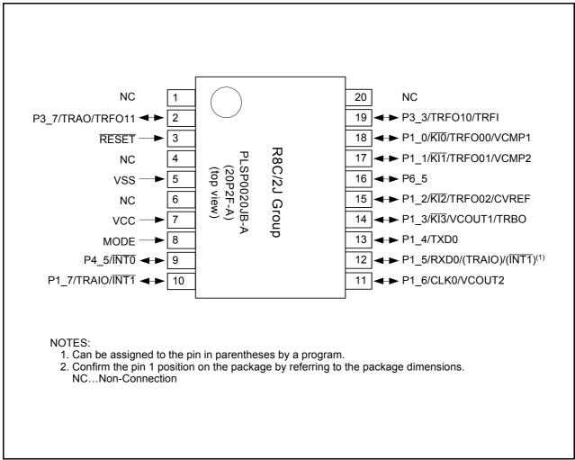
Figure 1.6 Pin Assignment (Top View) of R8C/2J Group
