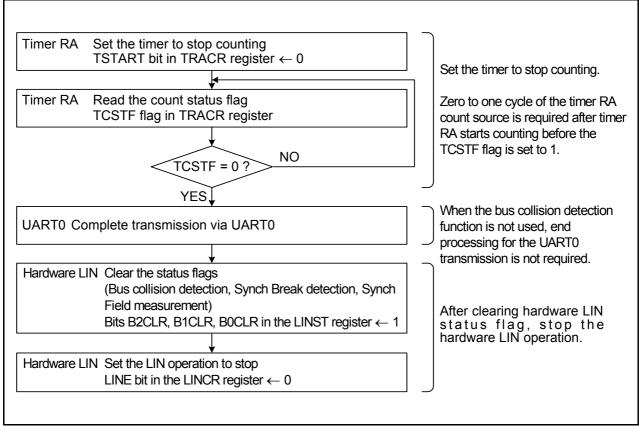
Figure 19.12 Example of Hardware LIN Communication Completion Flowchart
