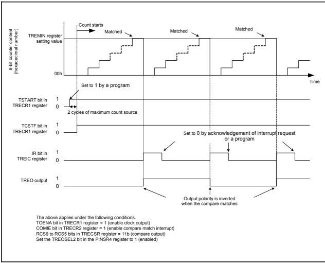
Figure 17.43 Operating Example in Output Compare Mode
