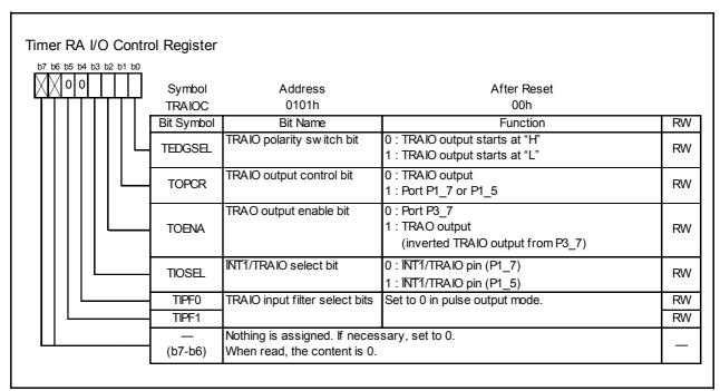
Figure 17.6 **TRAIOC Register in Pulse Output Mode**
