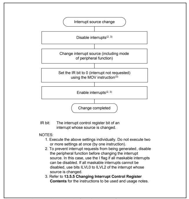
Figure 23.1 Example of Procedure for Changing Interrupt Sources
