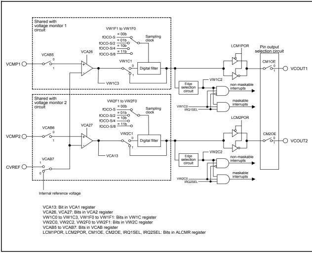
Figure 7.1 Block Diagram of Comparator
