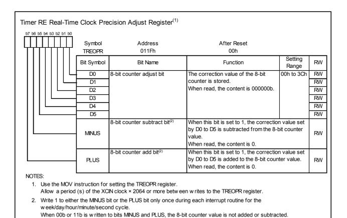
Figure 17.35 TREOPR Register in Real-Time Clock Mode
