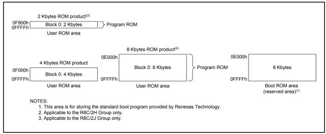
Figure 20.1 Flash Memory Block Diagram
