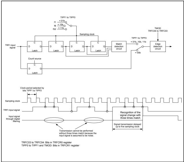
Figure 17.53 Block Diagram of Digital Filter
