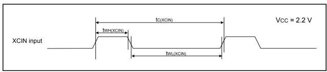
Figure 22.11 XCIN Input Timing Diagram when Vcc = 2.2 V
