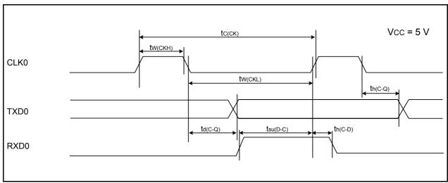
Figure 22.18 Serial Interface Timing Diagram when Vcc = 5 V
