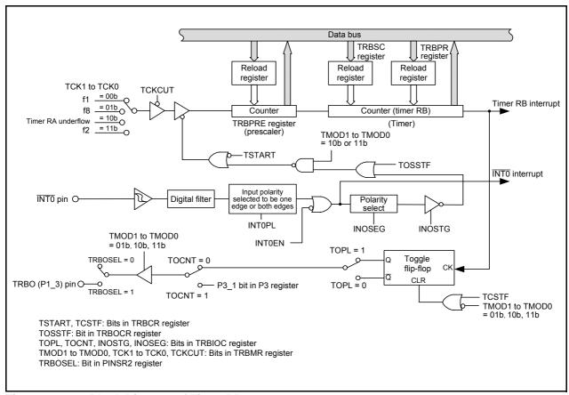
Figure 17.12 Block Diagram of Timer RB
