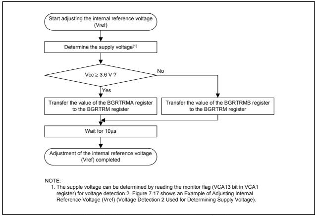
Figure 7.16 Procedure for Adjusting Internal Reference Voltage (Vref)
