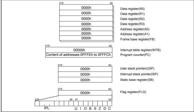
Figure 5.2 CPU Register Status after Reset
