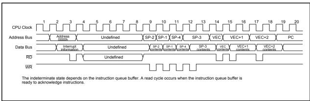
Figure 13.5 Time Required for Executing Interrupt Sequence
