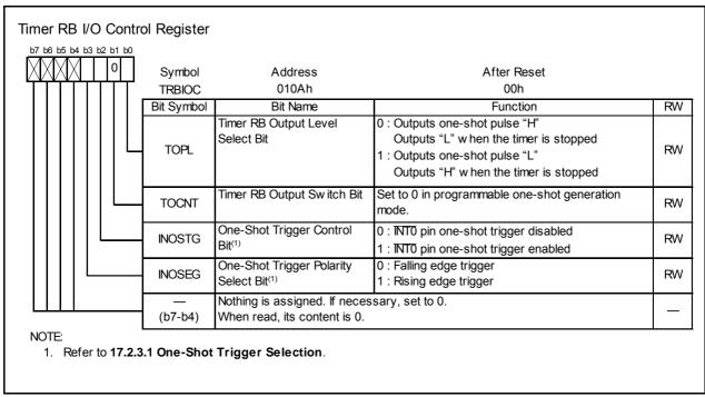
Figure 17.20 TRBIOC Register in Programmable One-Shot Generation Mode
