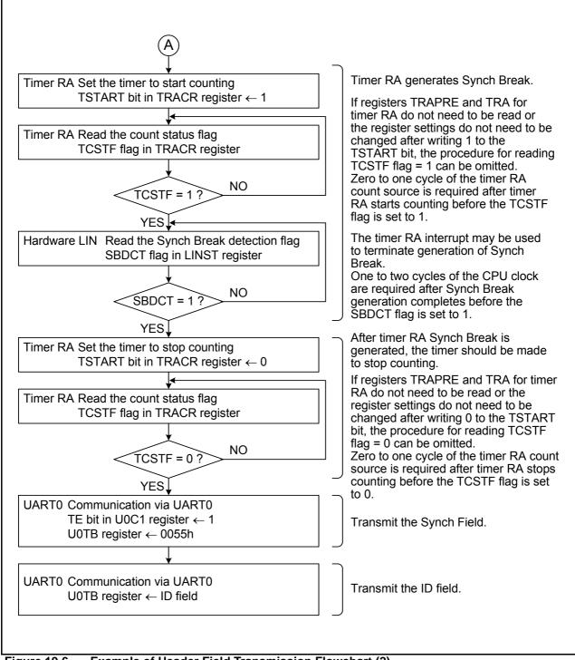
Figure 19.6 **Example of Header Field Transmission Flowchart (2)**
