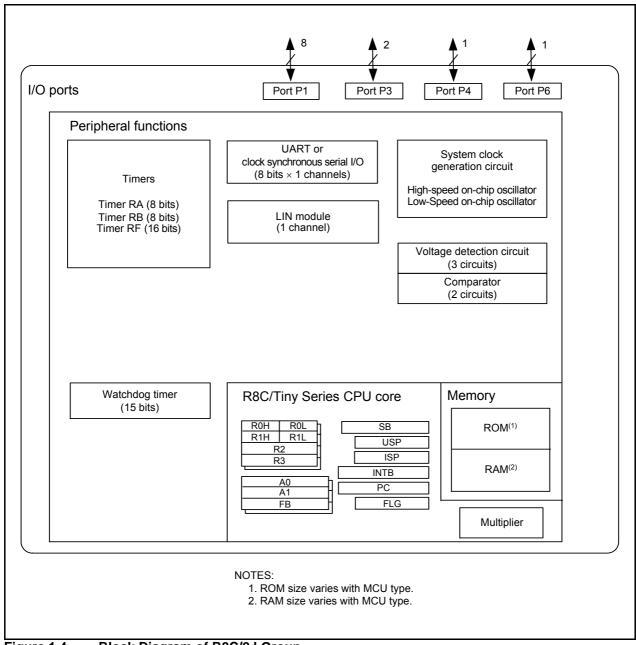
Figure 1.4 Block Diagram of R8C/2J Group
