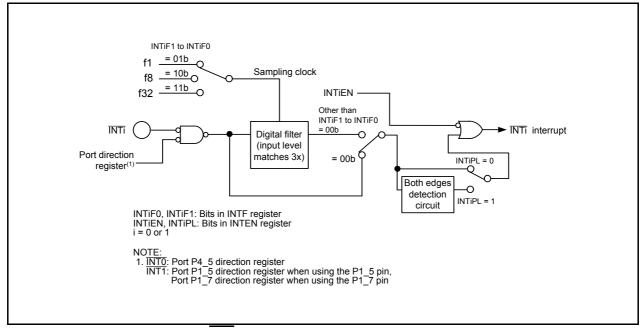
Figure 13.13 Configuration of INTi Input Filter
