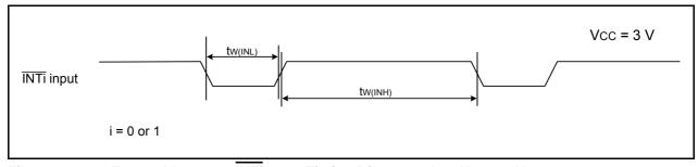
Figure 22.10 External Interrupt INTi Input Timing Diagram when Vcc = 3 V
