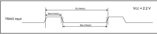
**Figure 22.23** TRAIO Input Timing Diagram when Vcc = 2.2 V
