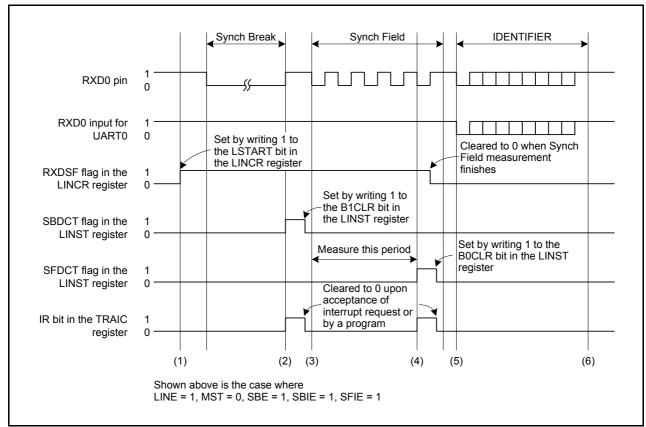
Figure 19.7 Typical Operation when Receiving a Header Field
