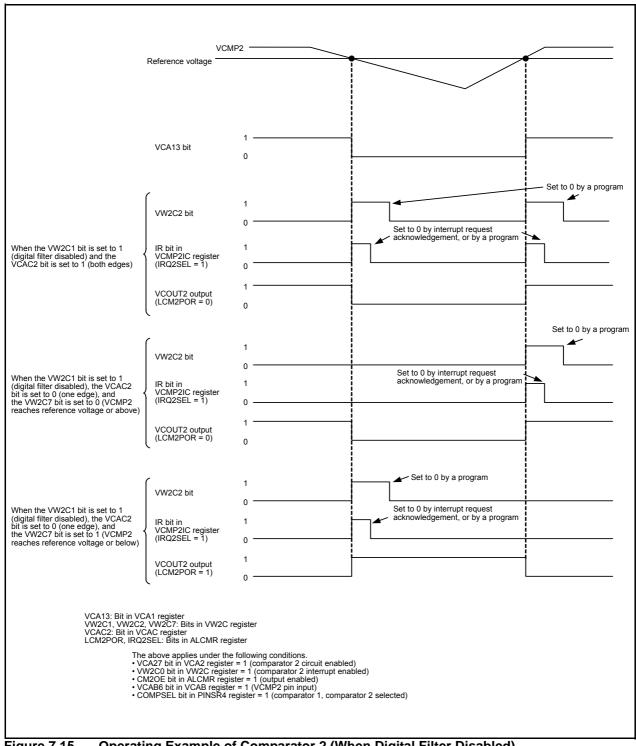
Operating Example of Comparator 2 (When Digital Filter Disabled) Figure 7.15
