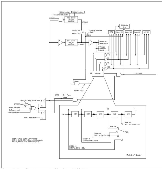
Figure 11.2 Clock Generation Circuit for R8C/2J Group
