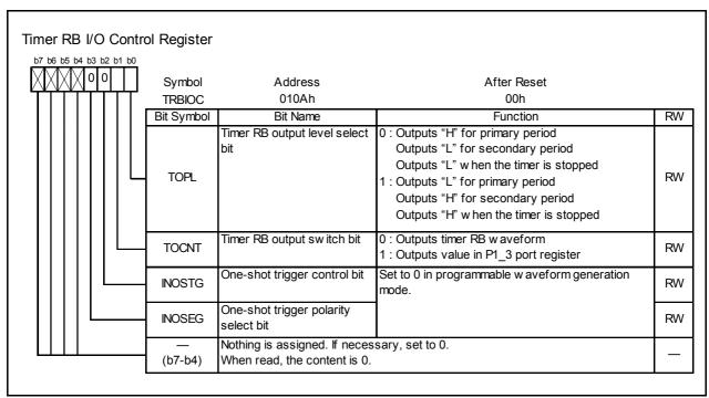
Figure 17.18 TRBIOC Register in Programmable Waveform Generation Mode
