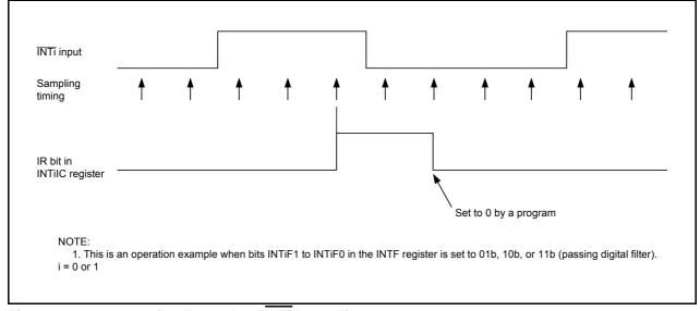
Figure 13.14 Operating Example of INTi Input Filter
