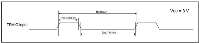
Figure 22.8 TRAIO Input Timing Diagram when Vcc = 3 V
