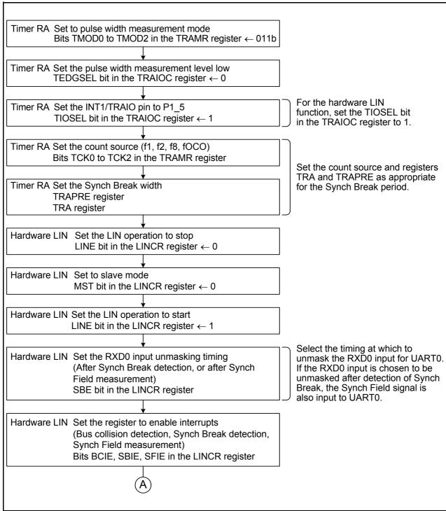
Figure 19.8 **Example of Header Field Reception Flowchart (1)**
