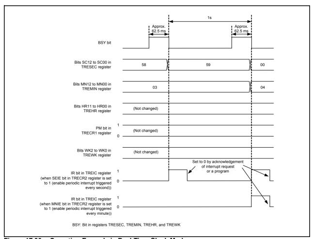
Figure 17.36 Operating Example in Real-Time Clock Mode
