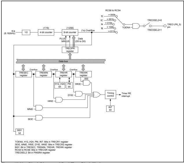
Figure 17.26 Block Diagram of Real-Time Clock Mode
