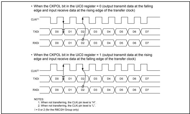
Figure 18.7 Transfer Clock Polarity
