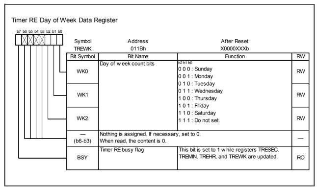
Figure 17.30 TREWK Register in Real-Time Clock Mode
