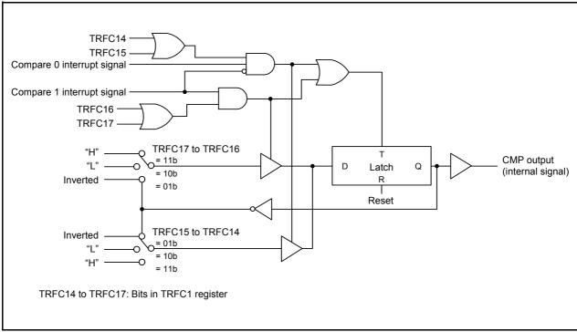
**Figure 17.46 Block Diagram of CMP Waveform Generation Unit**
