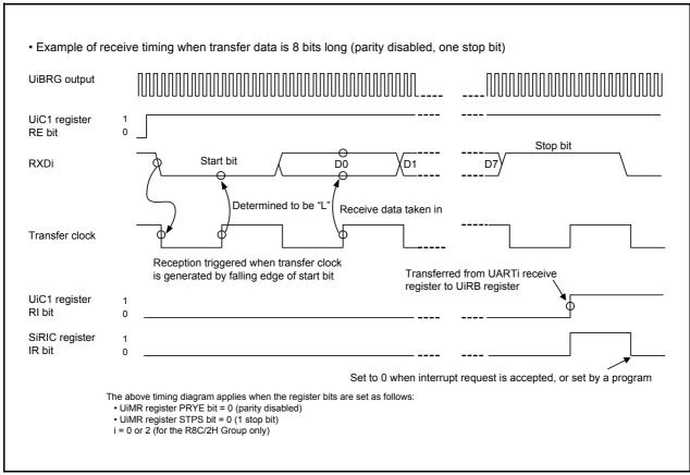
Figure 18.10 Receive Timing Example in UART Mode
