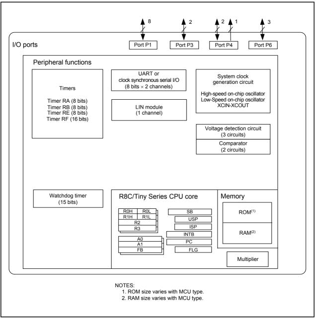
Figure 1.3 Block Diagram of R8C/2H Group
