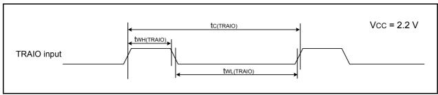
Figure 22.12 TRAIO Input Timing Diagram when Vcc = 2.2 V
