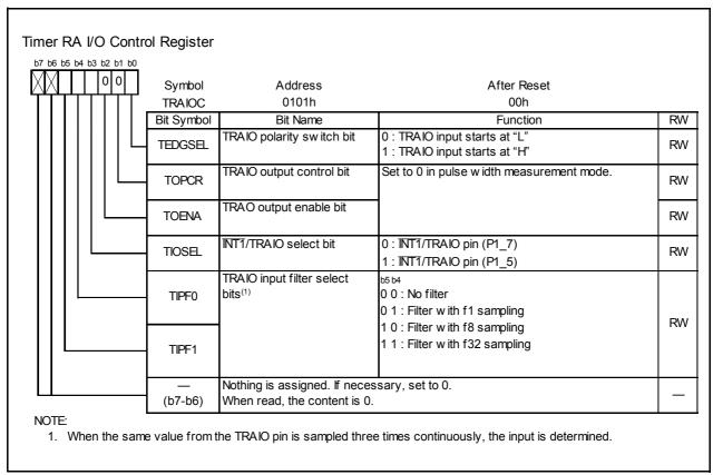
Figure 17.8 TRAIOC Register in Pulse Width Measurement Mode
