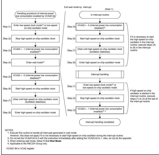
Figure 21.1 Handling Procedure of Internal Power Low Consumption Using VCA20 Bit
