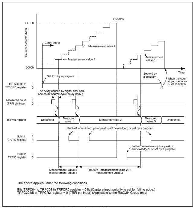
Figure 17.52 Operating Example in Input Capture Mode
