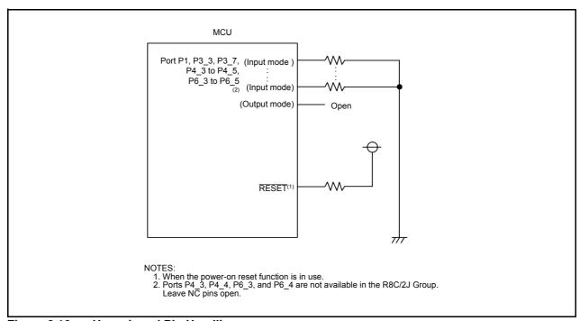
Figure 8.12 Unassigned Pin Handling
