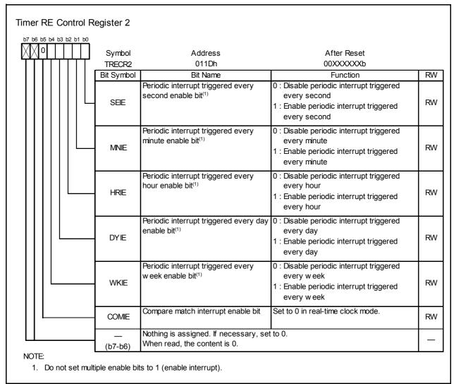
Figure 17.33 TRECR2 Register in Real-Time Clock Mode
