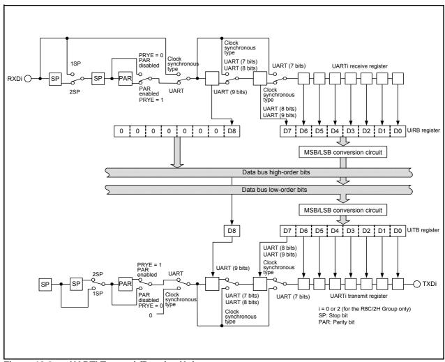
Figure 18.2 UARTi Transmit/Receive Unit
