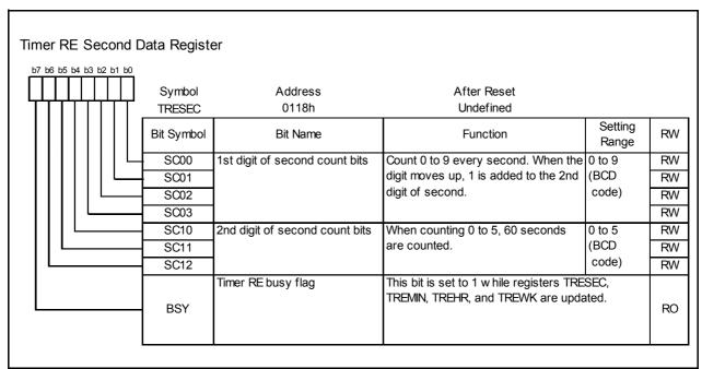
Figure 17.27 TRESEC Register in Real-Time Clock Mode
