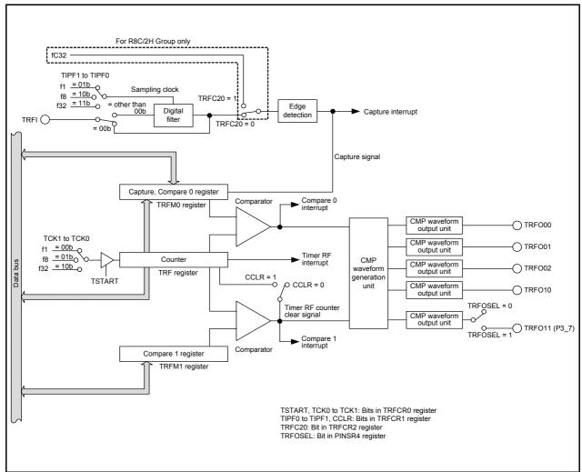
Figure 17.45 Block Diagram of Timer RF
