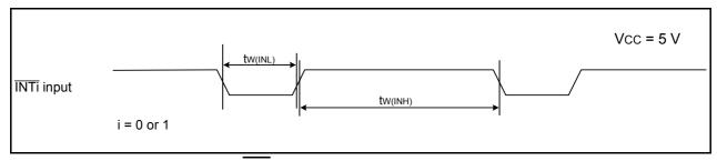
Figure 22.6 External Interrupt INTi Input Timing Diagram when Vcc = 5 V
