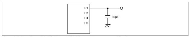
Figure 22.1 Ports P1, P3, P4, and P6 Timing Measurement Circuit
