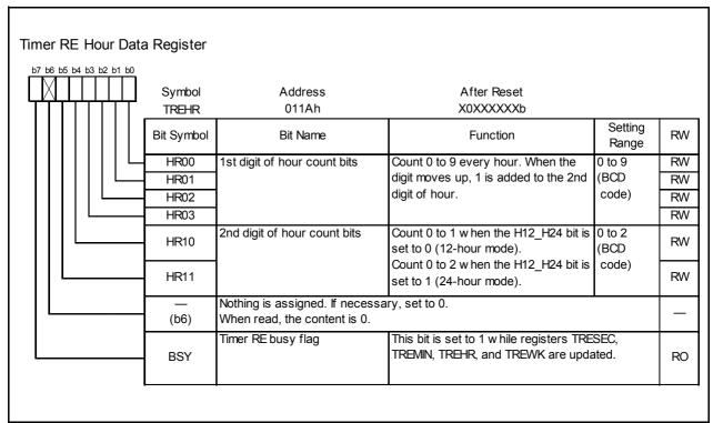
Figure 17.29 TREHR Register in Real-Time Clock Mode
