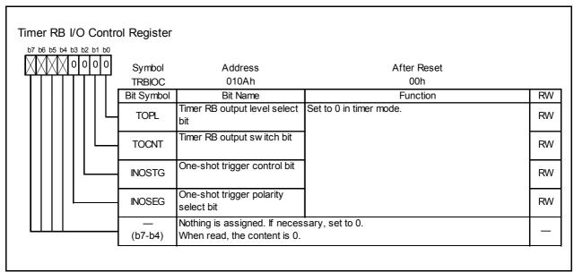
Figure 17.16 TRBIOC Register in Timer Mode
