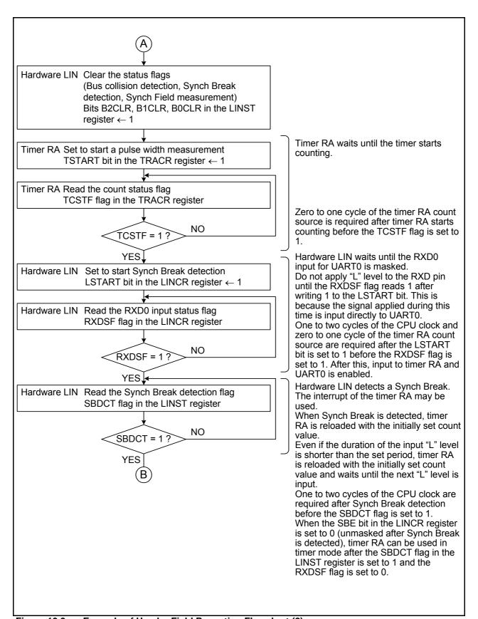
Figure 19.9 **Example of Header Field Reception Flowchart (2)**
