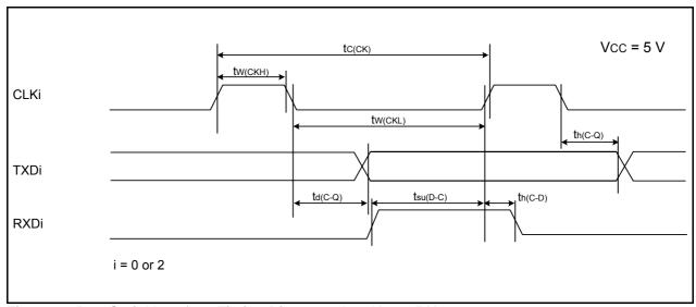
Figure 22.5 Serial Interface Timing Diagram when Vcc = 5 V
