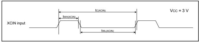
Figure 22.7 XCIN Input Timing Diagram when Vcc = 3 V
