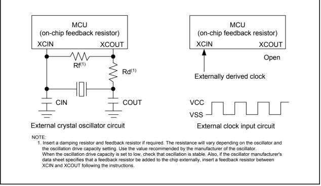
Figure 11.13 Examples of XCIN Clock Connection Circuits
