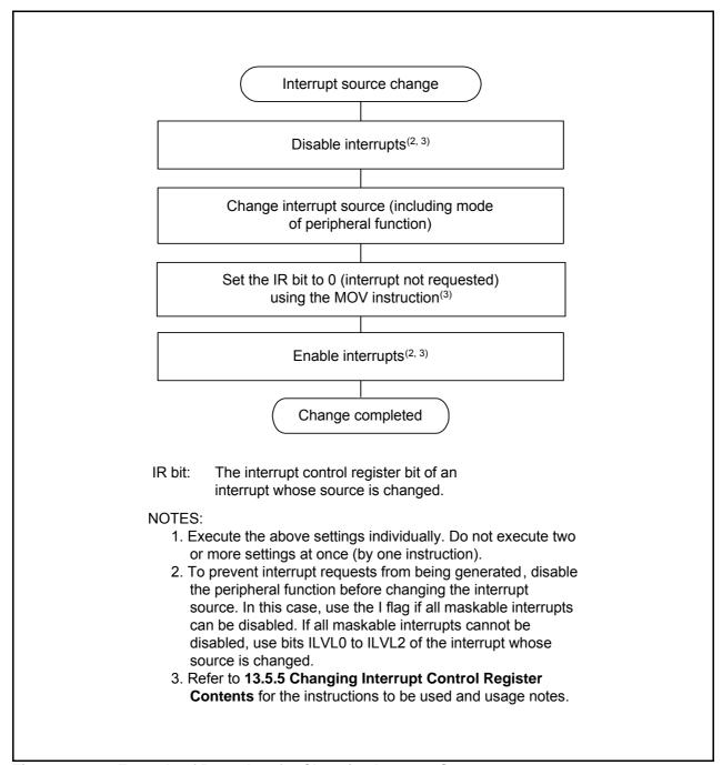
Figure 13.18 Example of Procedure for Changing Interrupt Sources
