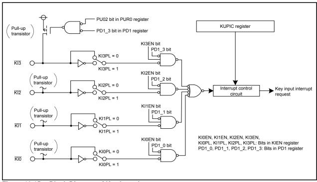
Figure 13.15 Block Diagram of Key Input Interrupt
