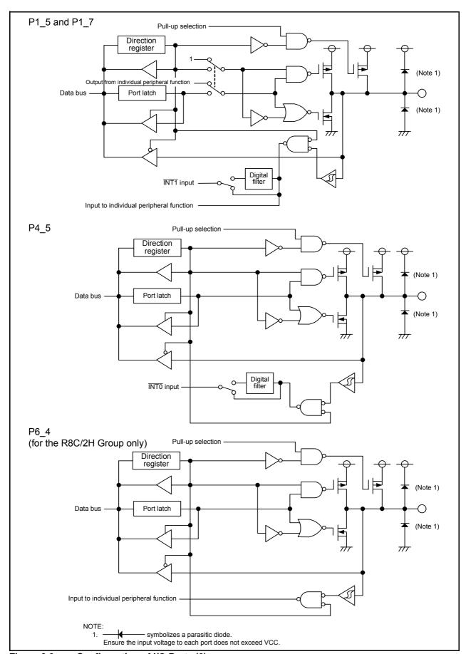
Figure 8.2 Configuration of I/O Ports (2)
