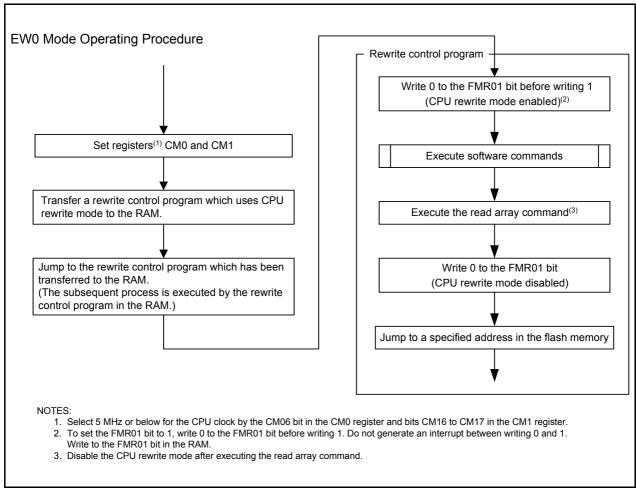
Figure 20.7 How to Set and Exit EW0 Mode
