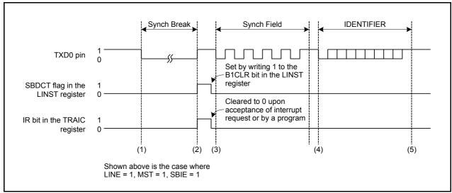
Figure 19.4 Typical Operation when Sending a Header Field
