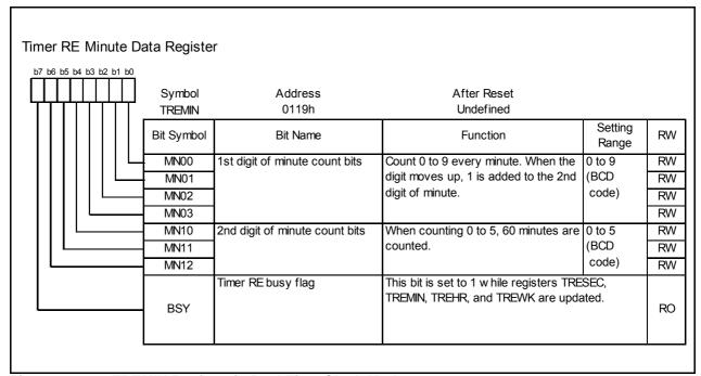
Figure 17.28 TREMIN Register in Real-Time Clock Mode
