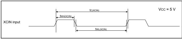
Figure 22.3 XCIN Input Timing Diagram when Vcc = 5 V
