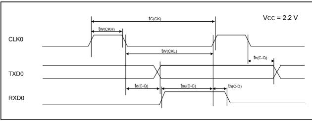
Figure 22.24 Serial Interface Timing Diagram when Vcc = 2.2 V
