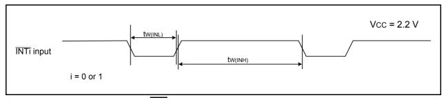
Figure 22.14 External Interrupt INTi Input Timing Diagram when Vcc = 2.2 V
