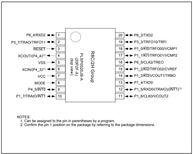
Figure 1.5 Pin Assignment (Top View) of R8C/2H Group
