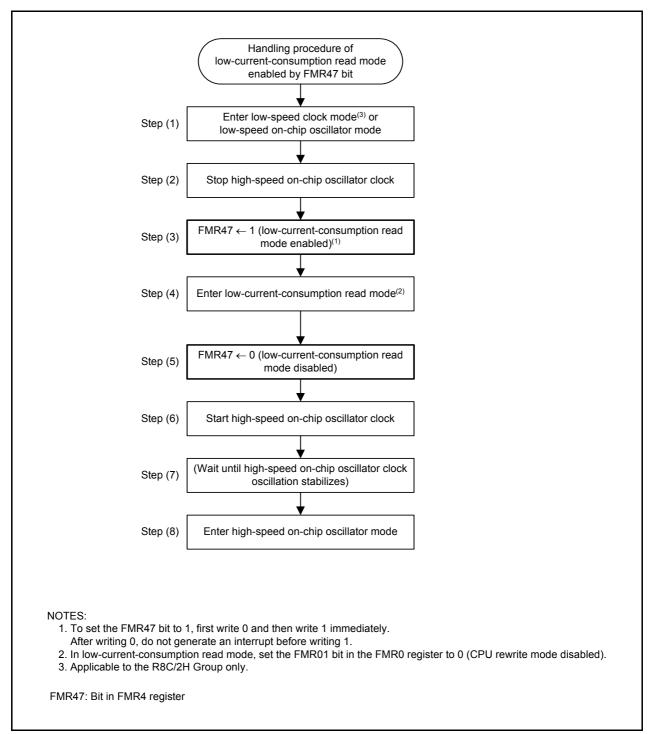
Figure 21.3 Handling Procedure Example of Low-Current-Consumption Read Mode
