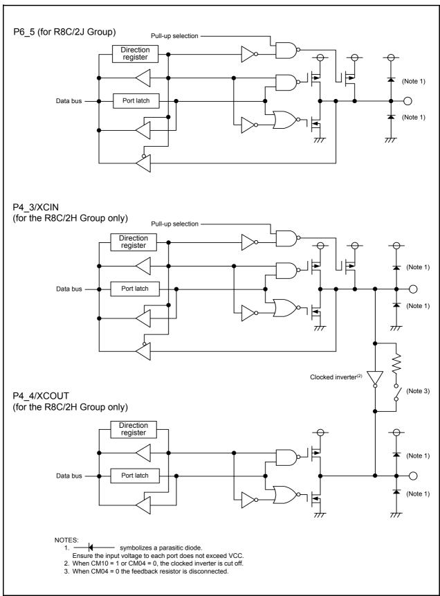
Figure 8.3 Configuration of I/O Ports (3)
