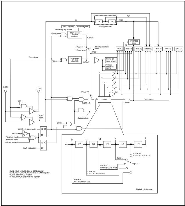
Figure 11.1 **Clock Generation Circuit for R8C/2H Group**
