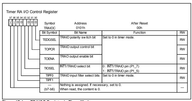
Figure 17.4 TRAIOC Register in Timer Mode
