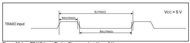
Figure 22.4 TRAIO Input Timing Diagram when Vcc = 5 V
