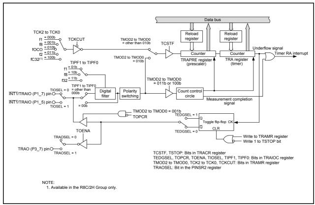
Figure 17.1 Block Diagram of Timer RA
