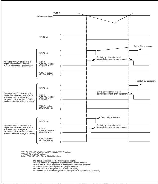
Operating Example of Comparator 1 (When Digital Filter Disabled) Figure 7.13
