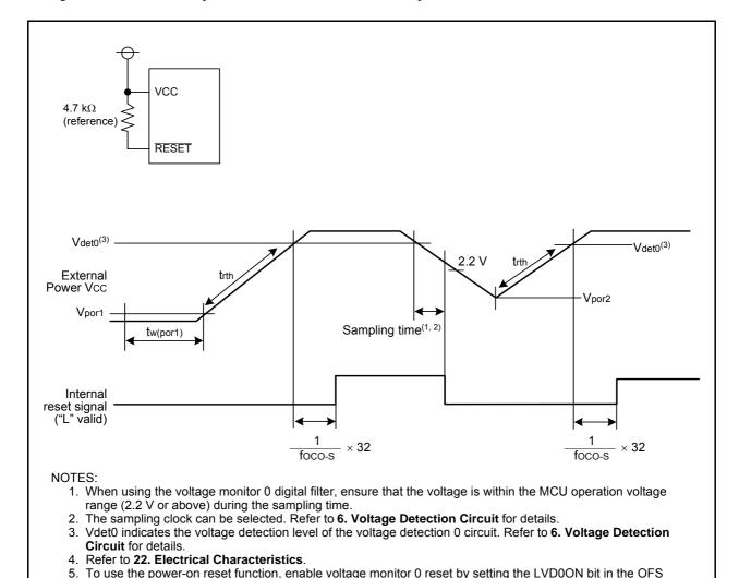
Figure 5.7 Example of Power-On Reset Circuit and Operation
