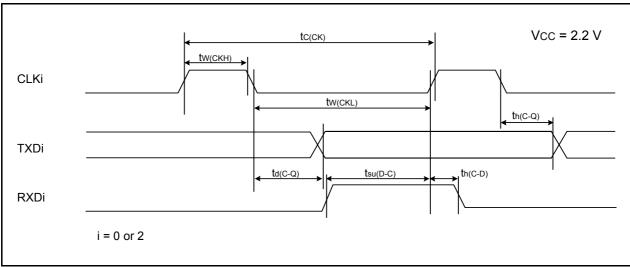
Figure 22.13 Serial Interface Timing Diagram when Vcc = 2.2 V
