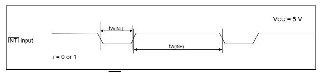
Figure 22.19 External Interrupt INTi Input Timing Diagram when Vcc = 5 V
