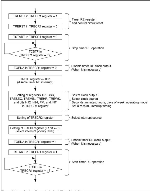
Figure 23.4 Setting Example in Real-Time Clock Mode
