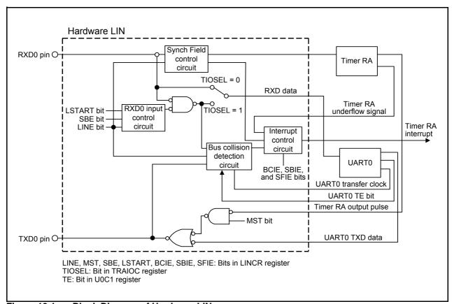
Figure 19.1 Block Diagram of Hardware LIN
