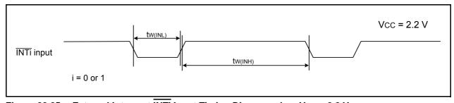
Figure 22.25 External Interrupt INTi Input Timing Diagram when Vcc = 2.2 V
