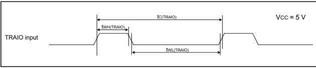
Figure 22.17 TRAIO Input Timing Diagram when Vcc = 5 V
