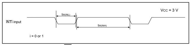
Figure 22.22 External Interrupt INTi Input Timing Diagram when Vcc = 3 V
