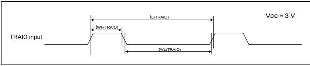
**Figure 22.20** TRAIO Input Timing Diagram when Vcc = 3 V
