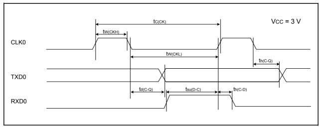
Figure 22.21 Serial Interface Timing Diagram when Vcc = 3 V
