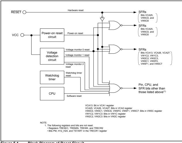
Figure 5.1 Block Diagram of Reset Circuit
