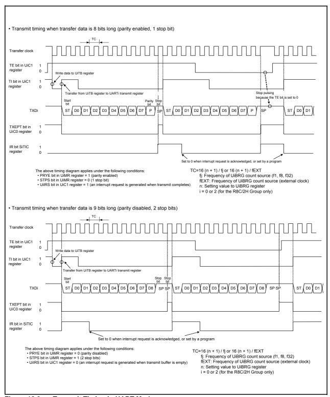
Figure 18.9 Transmit Timing in UART Mode
