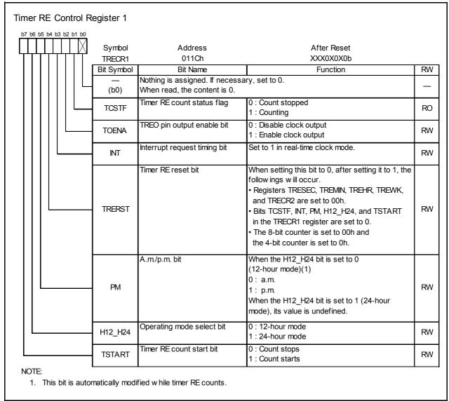
Figure 17.31 TRECR1 Register in Real-Time Clock Mode
