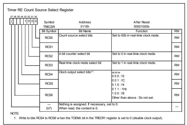
Figure 17.34 TRECSR Register in Real-Time Clock Mode
