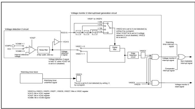
Block Diagram of Voltage Monitor 2 Interrupt/Reset Generation Circuit Figure 6.4
