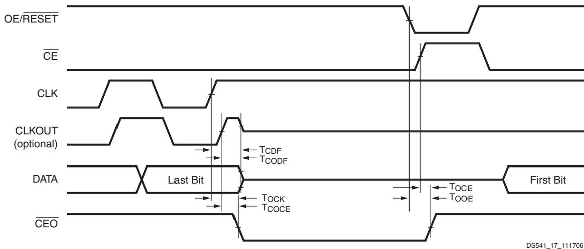
Figure 9: AC Characteristics Over Operating Conditions When Cascading
