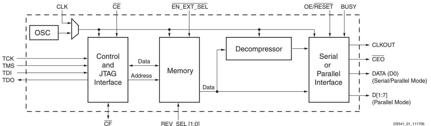
Figure 1: XQF32P Platform Flash PROM Block Diagram
