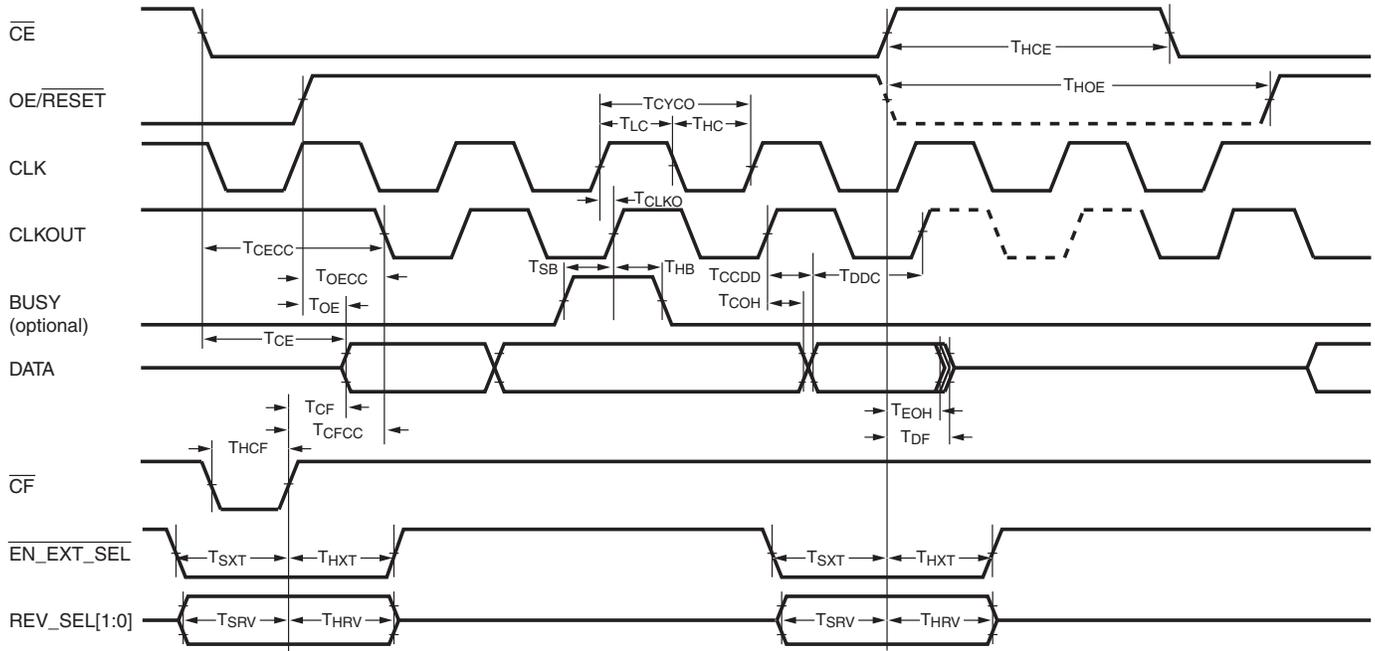
Note: 8 CLKOUT cycles are output after  $\overline{CE}$  rising edge, before CLKOUT is 3-stated, if OE/RESET remains High, and terminal count has not been reached.
