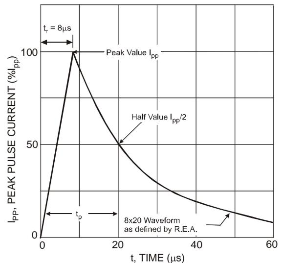
Fig. 2 Pulse Waveform
