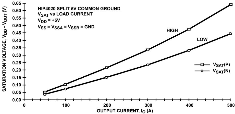
FIGURE 8. TYPICAL CHARACTERISTIC OF SATURATION VOLTAGE vs OUTPUT CURRENT USING A +5V SUPPLY, T<sub>AMBIENT</sub> = 25°C
