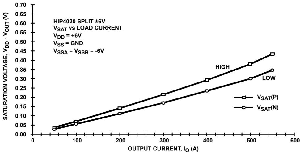
FIGURE 10. TYPICAL CHARACTERISTIC OF SATURATION VOLTAGE vs OUTPUT CURRENT USING A ±6V SPLIT SUPPLY, OUTPUT REFERENCE EQUAL LOGIC GROUND, T<sub>AMBIENT</sub> = 25°C
