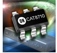
The CAT8710 is a space-saving, precision quad voltage supervisor, designed to monitor up to four supply voltages with a single device. When any supply voltage drops below its preset threshold, the CAT8710 will output a single reset to the threshold. One CAT8710 IC eliminates the need for multiple reset circuits, which minimizes system components and improves reliability.
