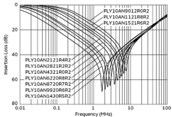
Differential Mode Insertion Loss-Frequency Characteristics
