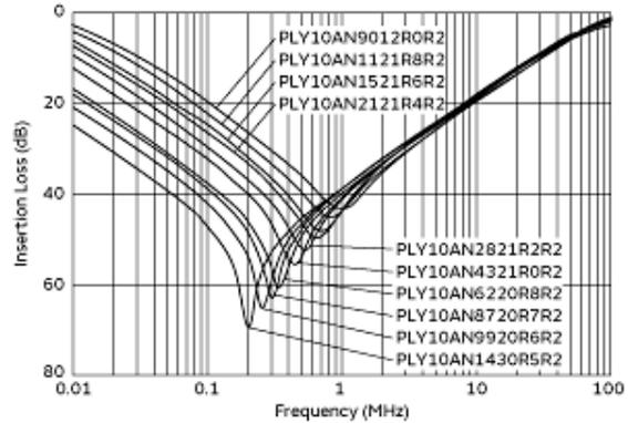
Common Mode Insertion Loss-Frequency Characteristics
