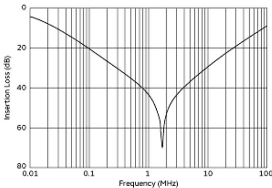
Differential Mode Insertion Loss (Typ.)
