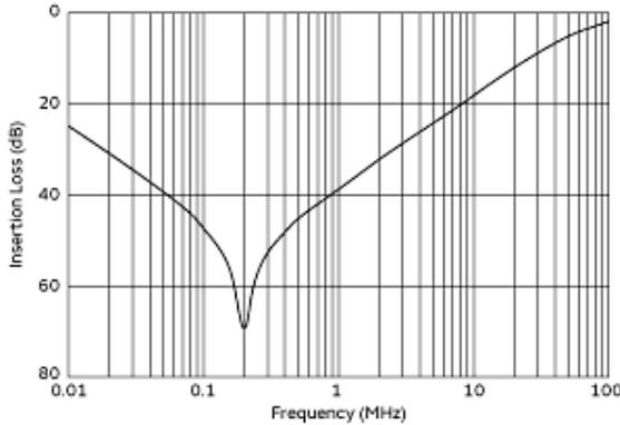
Common Mode Insertion Loss (Typ.)
