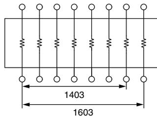
The 03 circuit provides a choice of 7 or 8 equal value resistors each connected between a common lead (14 or 16). Custom schematics available.
