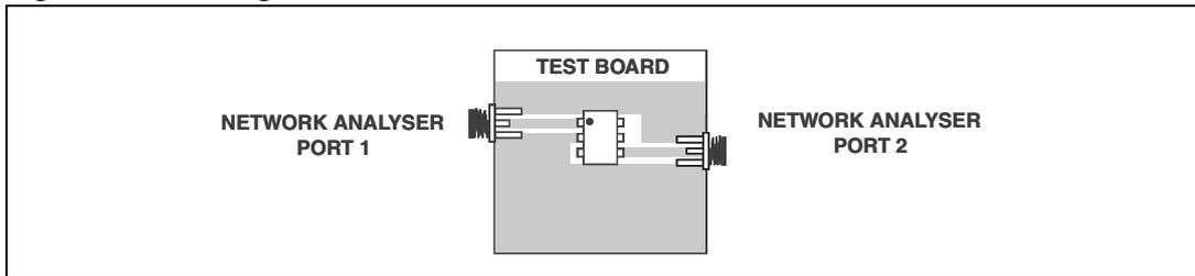
Figure 23 gives the measurement circuit for the analog application. In usual frequency range of analog signals (up to 240 MHz) the effect on disturbed line is less than -40 dB (see Figure 24 and Figure 25).
