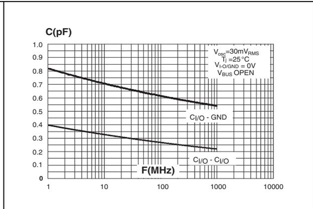
**Figure 4. Line capacitance versus frequency (typical values) HDMIULC6-2P6**
