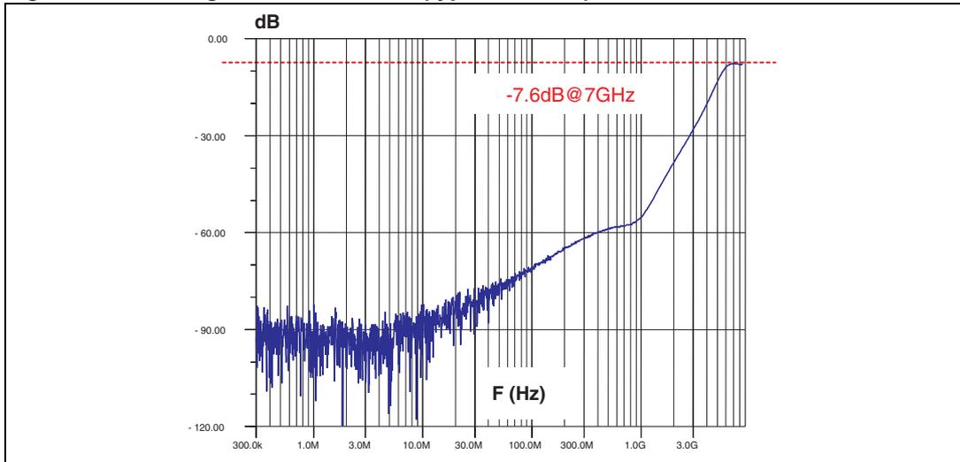
Figure 25. Analog crosstalk results (typical values) for HDMIULC6-2P6
