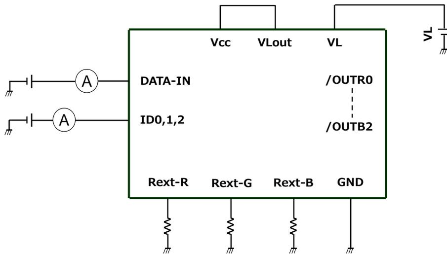
Test Circuit 2 Input Current (IIL)
