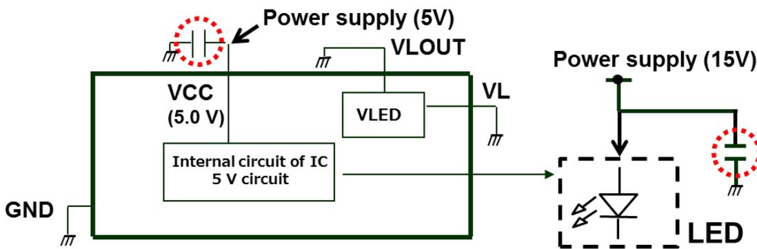
When 5V power supply is applied to this product without using the built-in power supply, ground VL pin and VLOUT pin.
