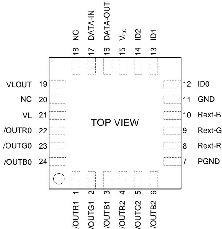
Please be sure to connect the back radiation PAD of a QFN package to GND of a substrate.
