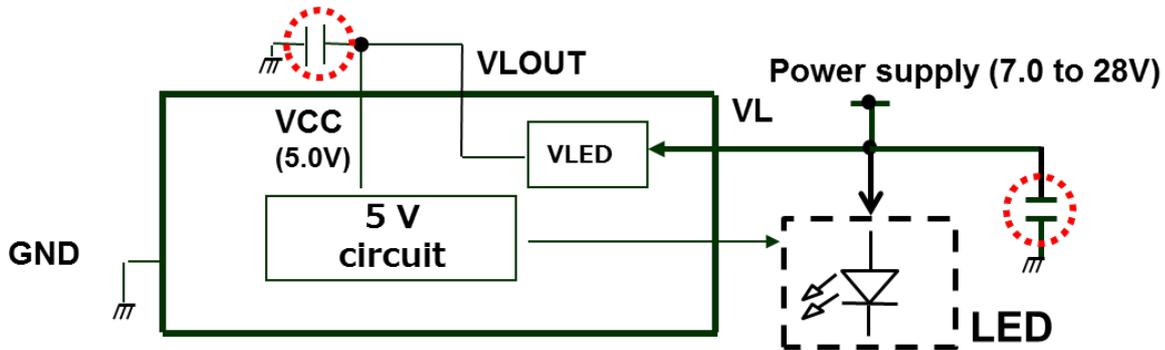
As shown in the above, the power supply (7.0 to 28V) is applied to the VL pin, and VLOUT and Vcc are connected directly. Connect VLOUT pin output (5V) to Vcc of own product, and also only 1 pcs of logic IC. (Do not connect with two or more logic ICs or other LED drivers.)
