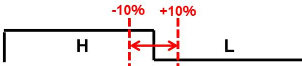
If there is no reversal of data polarity in this window, data cannot be recognized.
