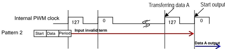
Outputting data A does not start at the rising edge of zero internal PWM clock just after the data A is input. It starts at the next rising edge of zero internal PWM clock. Inputting is invalid from the data A (period) input to the rising edge of after the next zero internal PWM clock.
