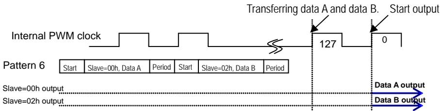
Both data A and data B are output at the rising edge of zero internal PWM clock which is just after the data A and the data B inputs.
