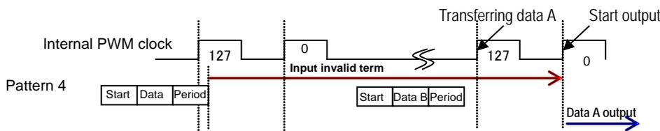
Inputting is invalid from the data A (period) input to the rising edge of the second internal clock. So, data B is invalid and data A is output.
