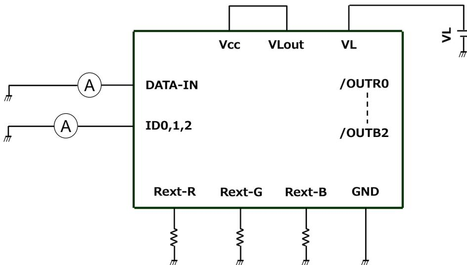
Test Circuit 3 Supply Current (VL)
