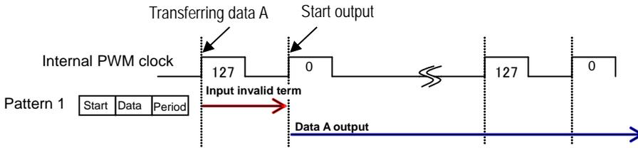
Output data A starts at the rising edge of zero internal PWM clock. Inputting is invalid from the rising edge of 127 internal PWM clocks to the rising edge of zero internal PWM clock which is just after these 127 PWM clocks.
