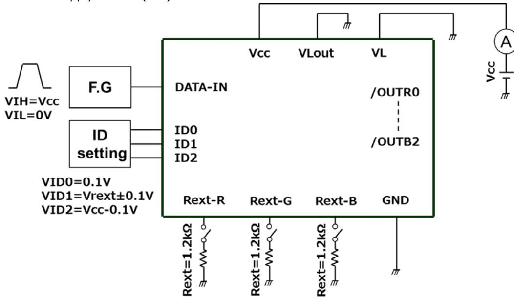
Test Circuit5 Output Current/ Output Leakage Current/ Output Current Accuracy/ Changes in Constant Output current dependent on Vcc
