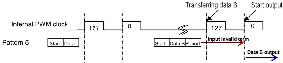
Outputting data A does not start at the rising edge of zero internal clock which is just after the data A input. Outputting data B starts at the rising edge of zero internal PWM clock which is just after the data B input.
