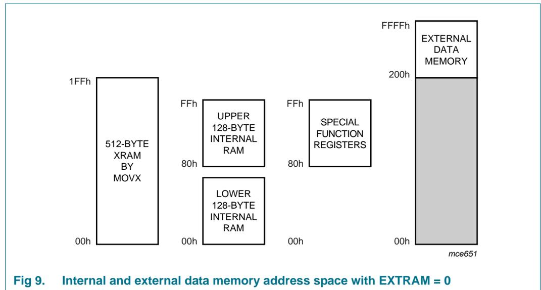
Fig 9. Internal and external data memory address space with EXTRAM = 0
