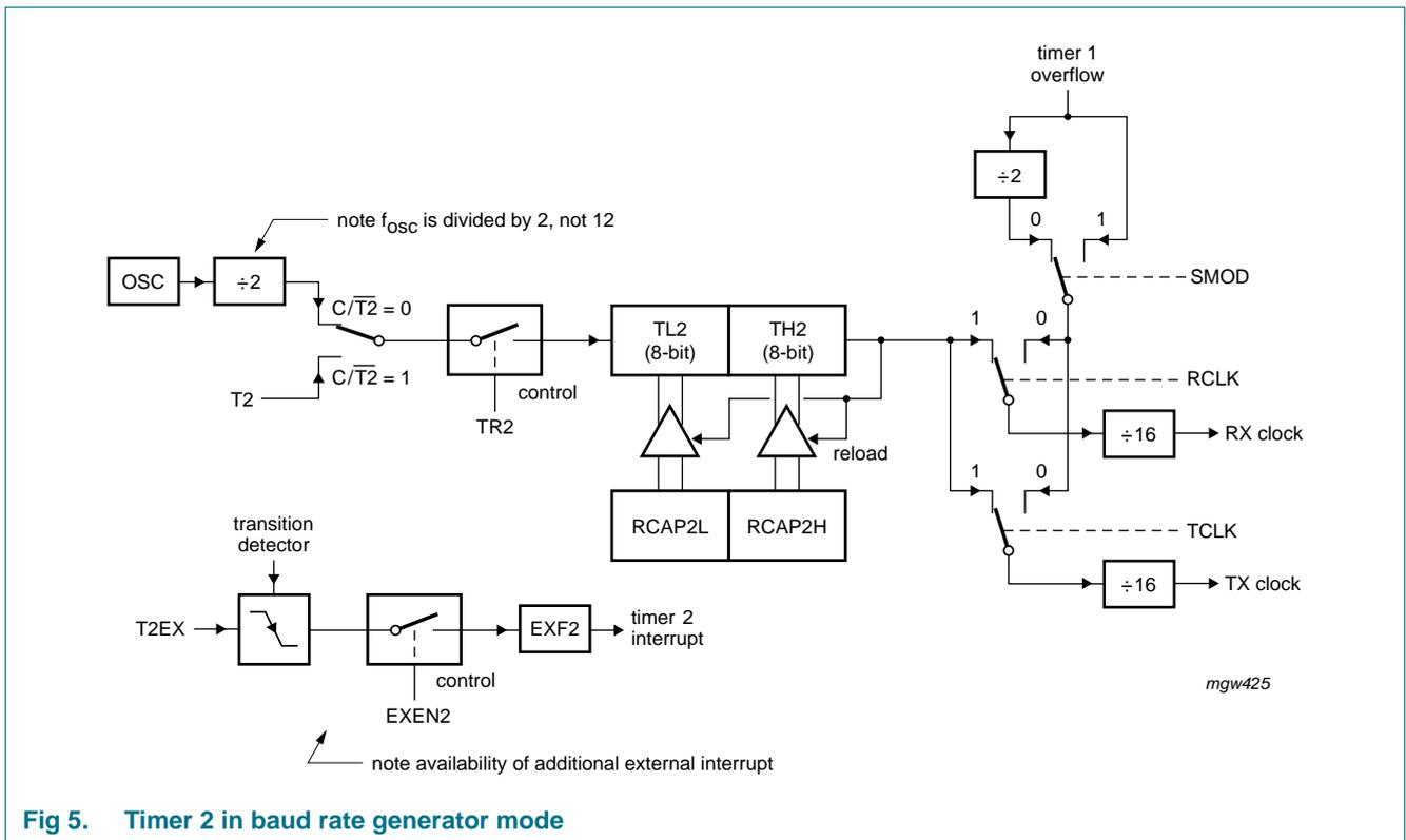
Fig 5. Timer 2 in baud rate generator mode
