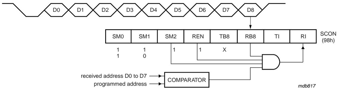
UART modes 2 or 3 and SM2 = 1: there is an interrupt if REN = 1, RB8 = 1 and received address is equal to programmed address.
