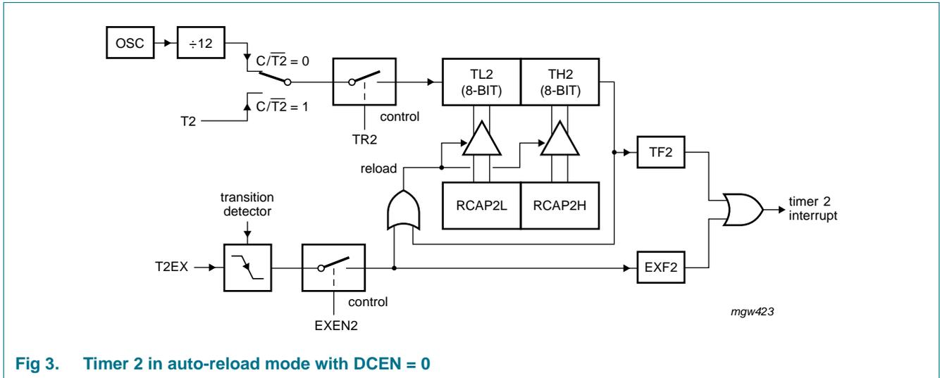
Fig 3. Timer 2 in auto-reload mode with DCEN = 0
