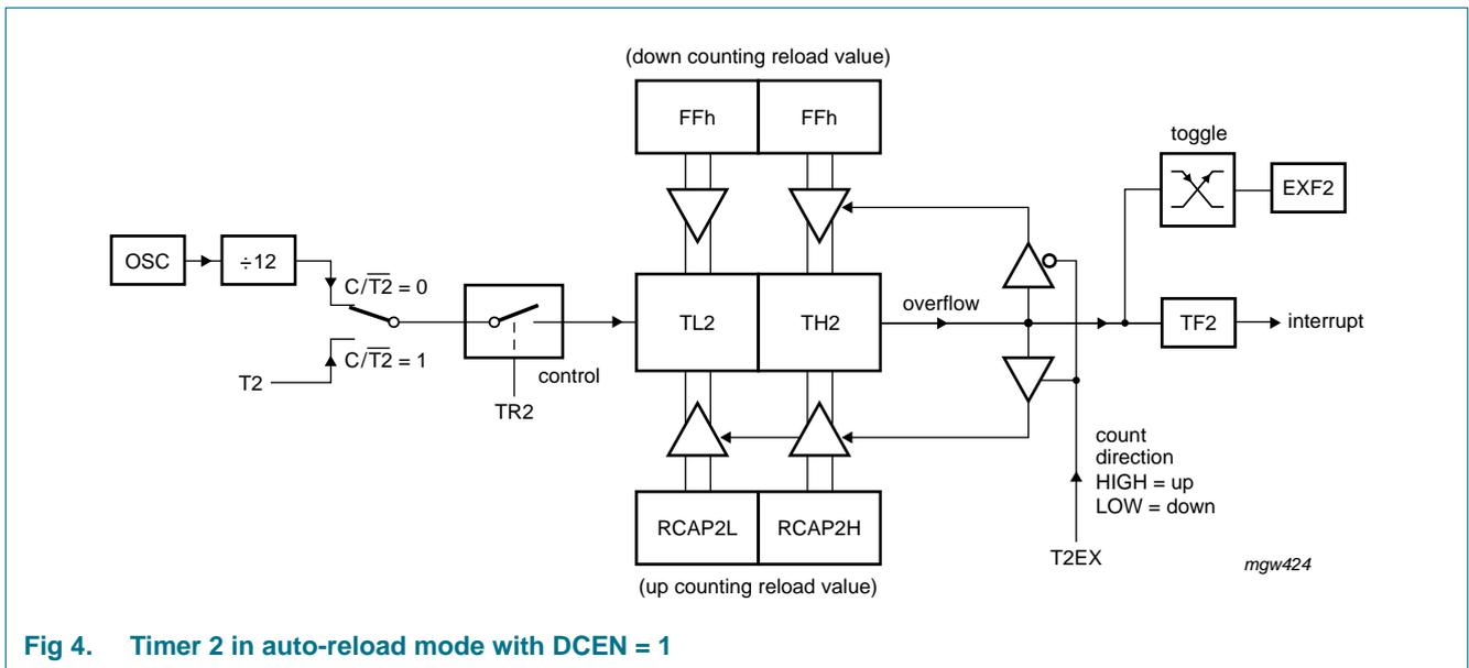
Fig 4. Timer 2 in auto-reload mode with DCEN = 1
