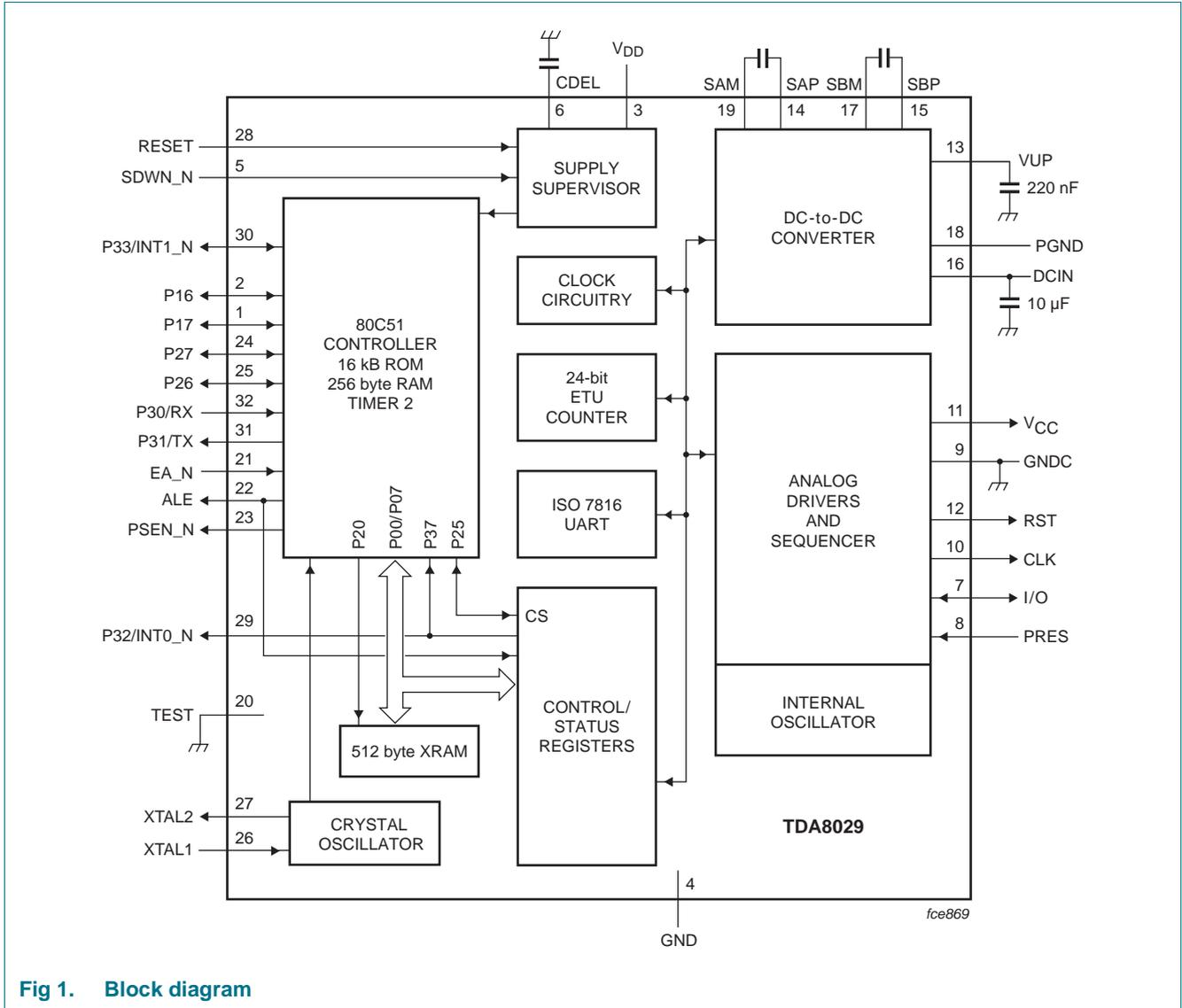
Fig 1. Block diagram
