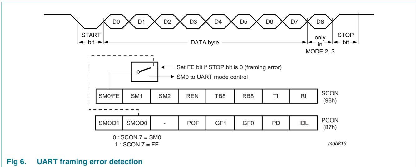
**Fig 6. UART framing error detection**
