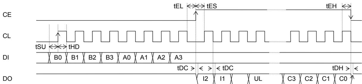
Note: Since the DO pin is an N-channel open-drain pin, the time for the data to change ( $t_{DC}$  and  $t_{DH}$ ) will differ depending on the value of the pull-up resistor and printed circuit board capacitance.
