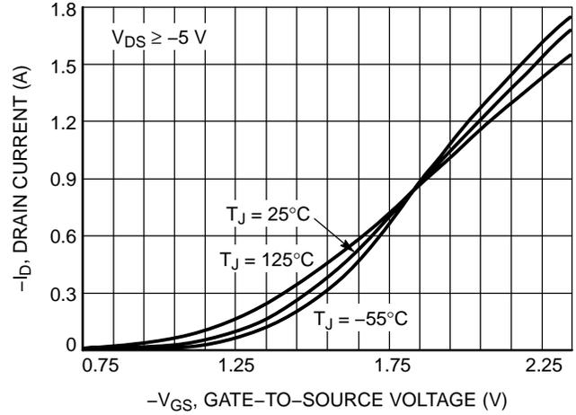
Figure 2. Transfer Characteristics
