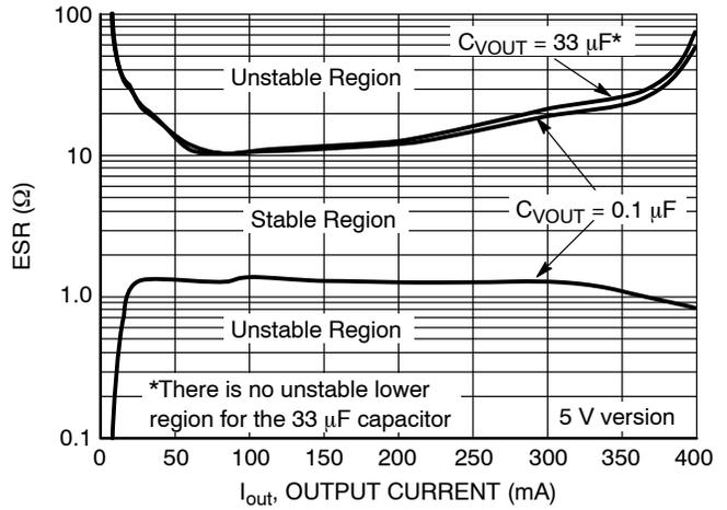
Figure 10. Output Stability with Output Capacitor Change
