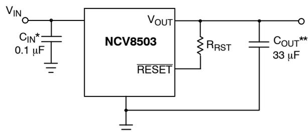
\* $C_{IN}$  required if regulator is located far from the power supply filter
