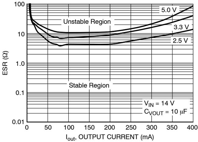
Figure 9. Output Stability with Output Voltage Change
