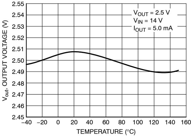
Figure 5. 2.5 V Output Voltage vs. Temperature
