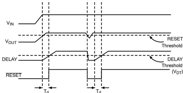
Figure 15. Reset and Delay Circuit Wave Forms
