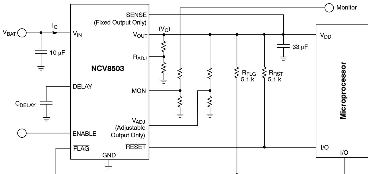
Figure 1. Application Diagram
