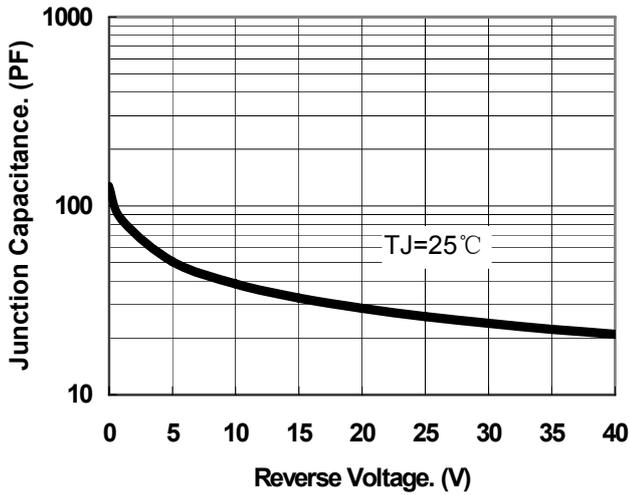
Fig.1-Typical Junction Capacitance
