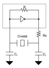
$$\begin{split} C_L &= 2^*(C_P - C_S),\\ \text{Where } C_P &= \text{Load capacitance of crystal.}\\ C_S &= \text{Stray capacitance due to } C_{\text{IN,}} \text{ PCB, Trace, etc.} \end{split}$$
