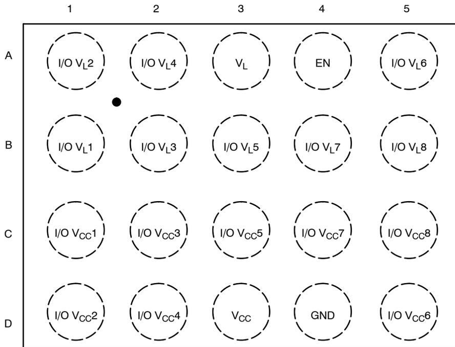
**Figure 3. 20 Flip-Chip (2.54 mm x 2.03 mm)**
