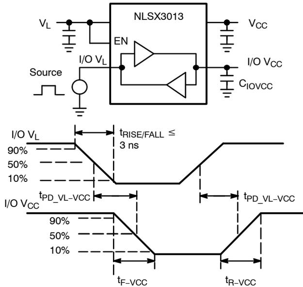
Figure 4. Driving I/O V<sub>L</sub> Test Circuit and Timing
