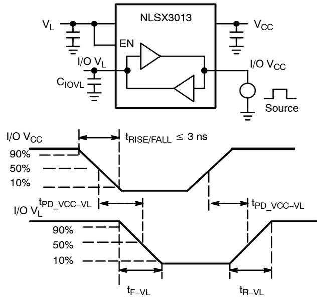
Figure 5. Driving I/O V<sub>CC</sub> Test Circuit and Timing
