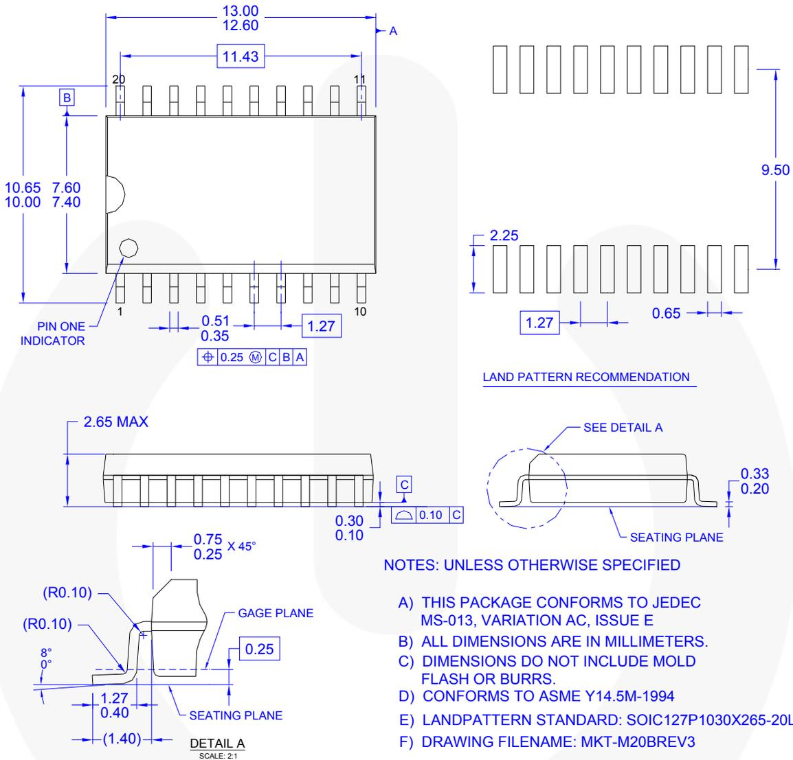
Figure 49. 20-Pin, Small-Outline Integrated Circuit (SOIC) Package
