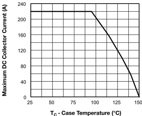
Fig. 3 - Maximum Collector Current vs. Case Temperature
