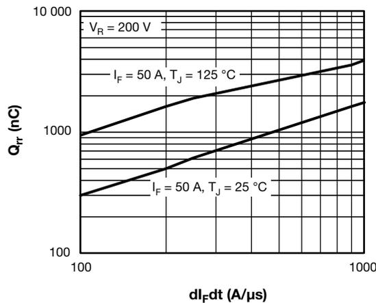
Fig. 11 - Typical Stored Charge vs.  $dI_F/dt$
