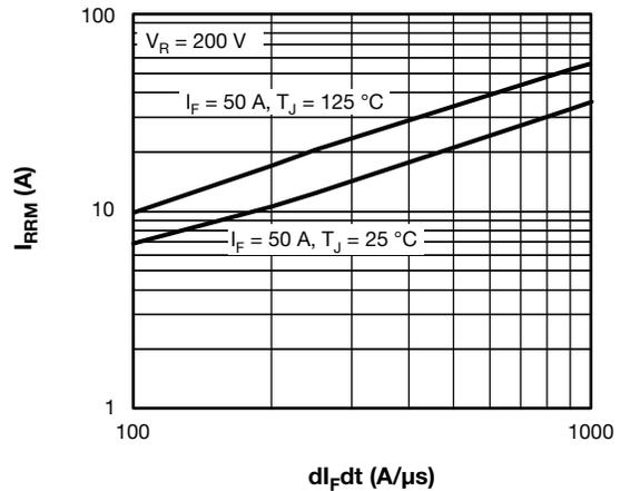
Fig. 10 - Typical Reverse Recovery Current vs.  $dI_F/dt$
