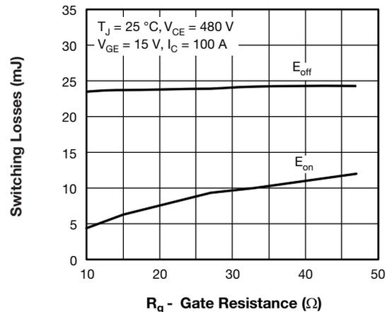
Fig. 6 - Typical Switching Losses vs. Gate Resistance
