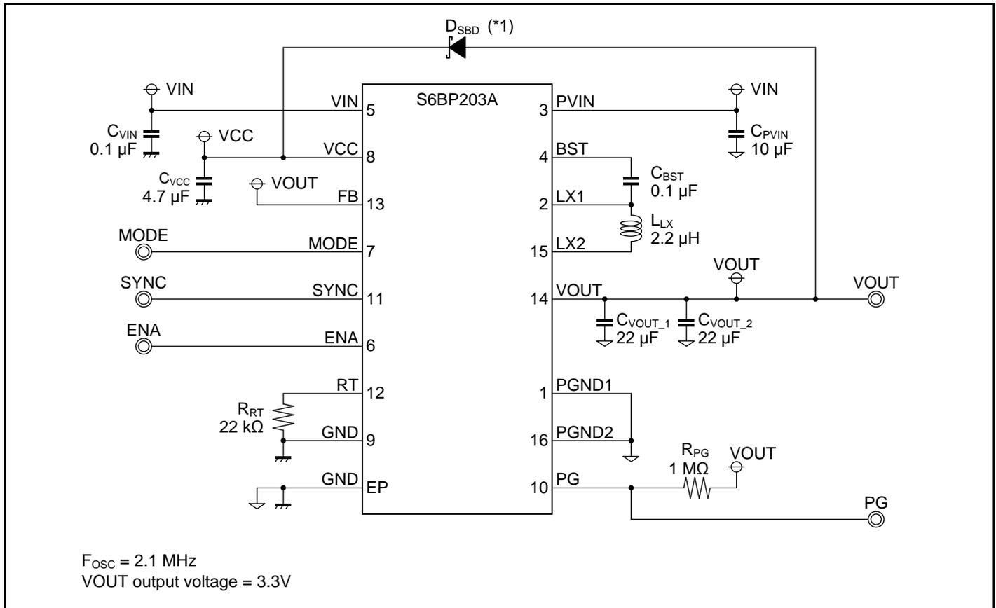
\*1: The  $D_{SBD}$  is necessary only when using at  $V_{IN} \leq 3.3\text{V}$ . In addition, since a leakage current ( $I_R$ ) of the  $D_{SBD}$  increases under high temperature, it is necessary to connect a load according to the leakage current of the  $D_{SBD}$  to  $V_{OUT}$  pin under the automatic PWM/PFM switching operation (MODE = L, SYNC = L).
