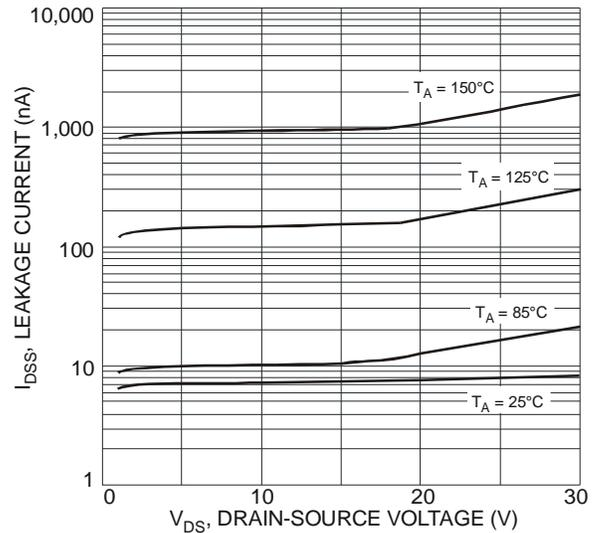
Fig. 13 Typical Leakage Current vs. Drain-Source Voltage
