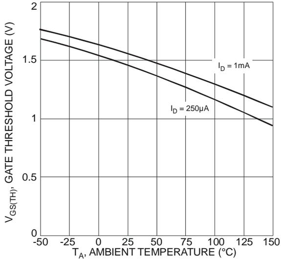
Fig. 10 Gate Threshold Variation vs. Ambient Temperature
