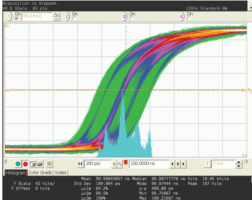
10MHz output clock from Jitter Attenuator - 75ps peak-to-peak period jitter
