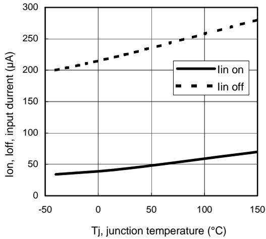
**Figure 13 – Input current (µA) On and Off
