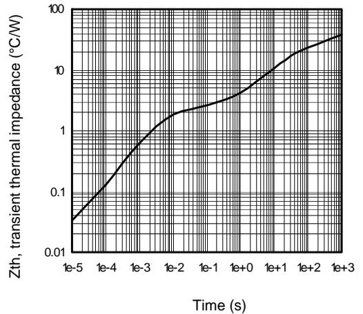
**Figure 12 – Transient thermal impedance (°C/W) Vs time (s)**
