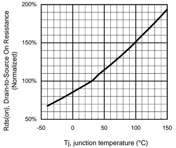
Figure 6 – Normalized Rds(on) (%) Vs Tj (°C)
