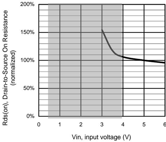
Figure 5 – Normalized Rds(on) (%) Vs Input voltage (V)
