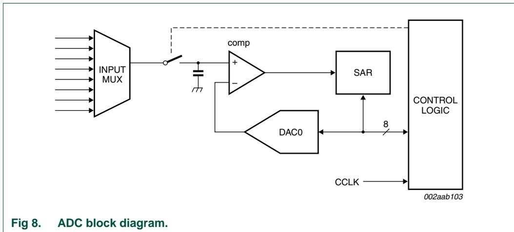
Fig 8. ADC block diagram.
