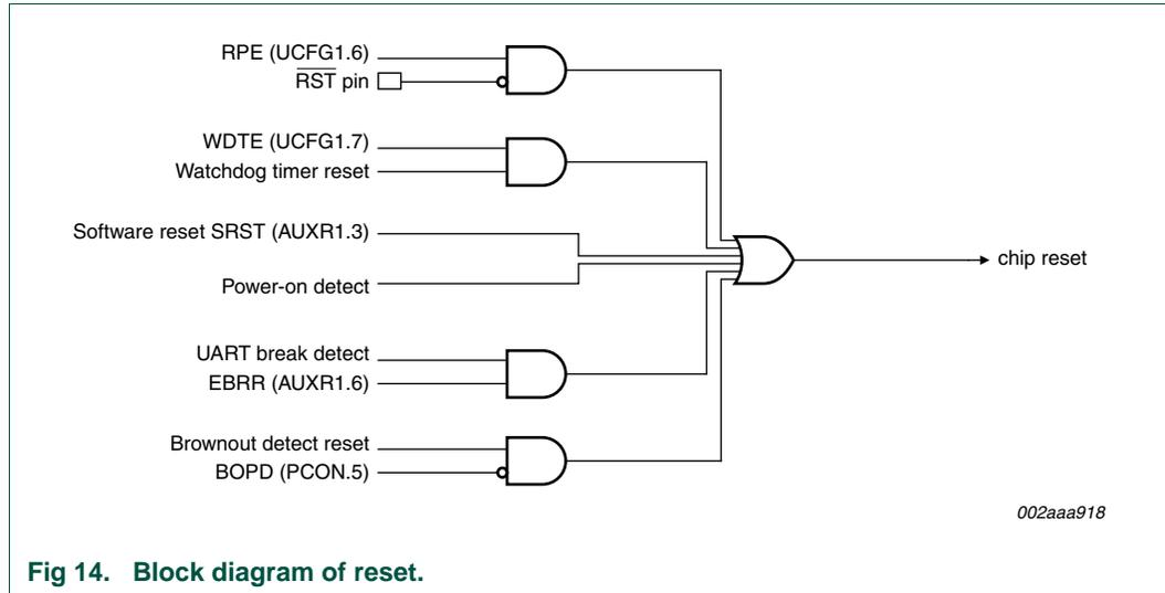
Fig 14. Block diagram of reset.
