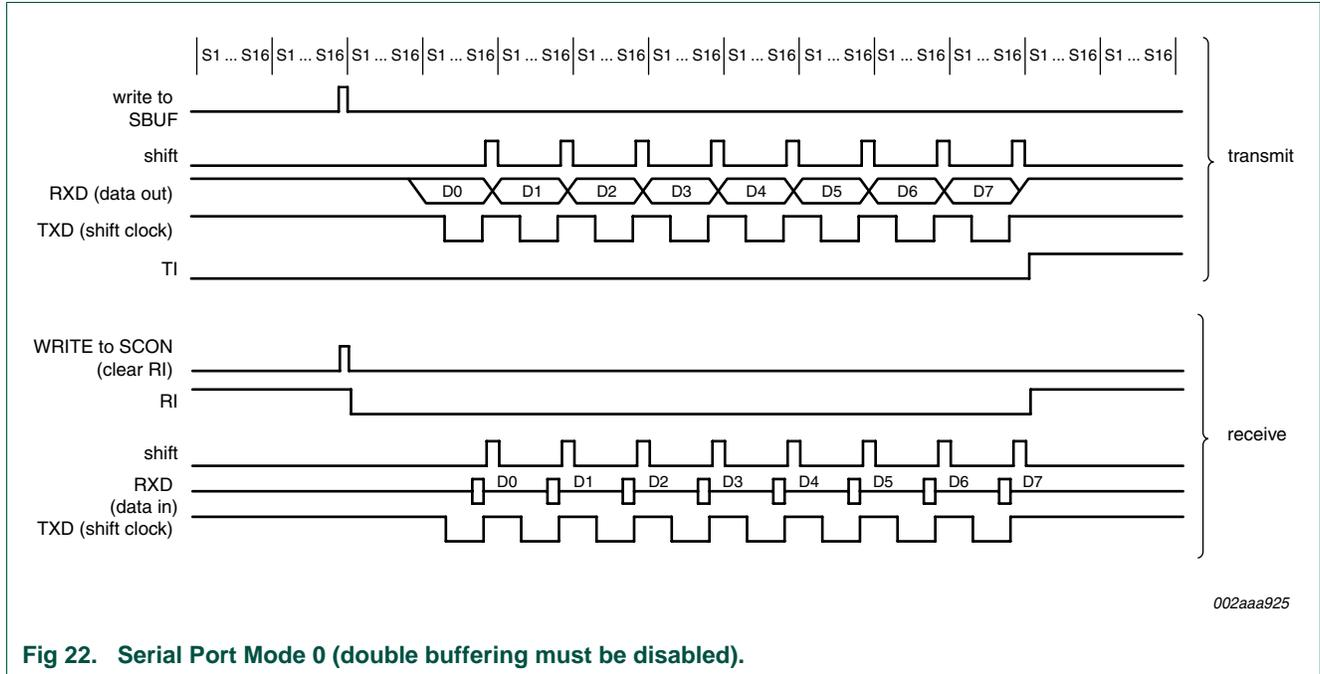
Fig 22. Serial Port Mode 0 (double buffering must be disabled).
