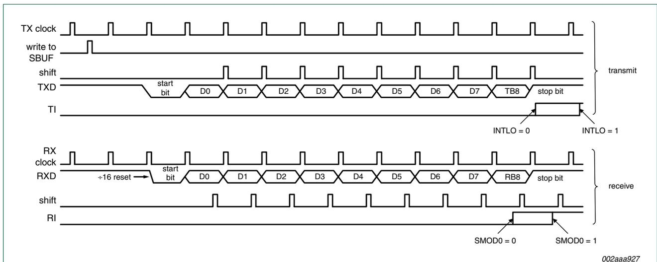
Fig 24. Serial Port Mode 2 or 3 (only single transmit buffering case is shown).
