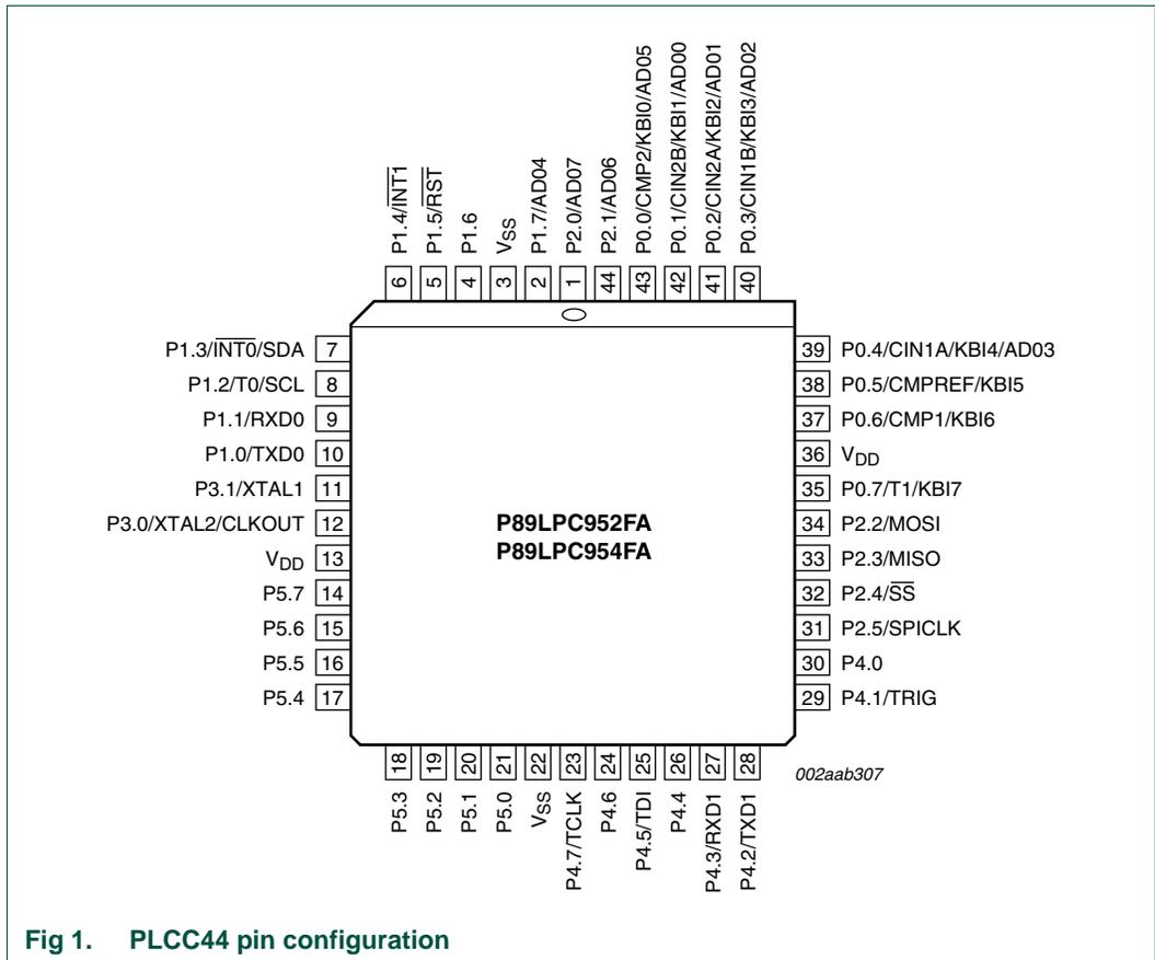
Fig 1. PLCC44 pin configuration
