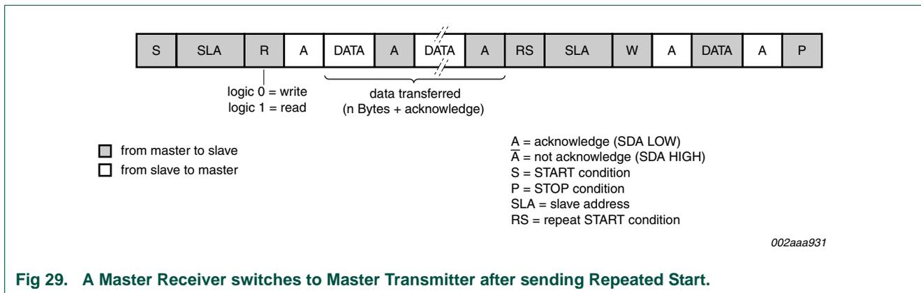
**Fig 29. A Master Receiver switches to Master Transmitter after sending Repeated Start.**
