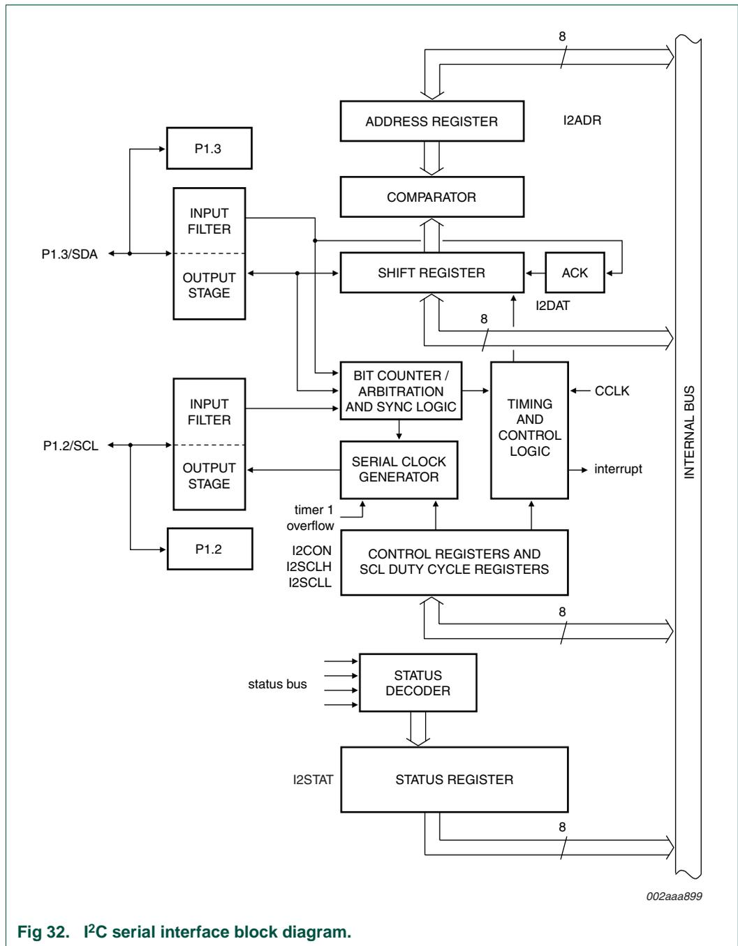
Fig 32. I<sup>2</sup>C serial interface block diagram.
