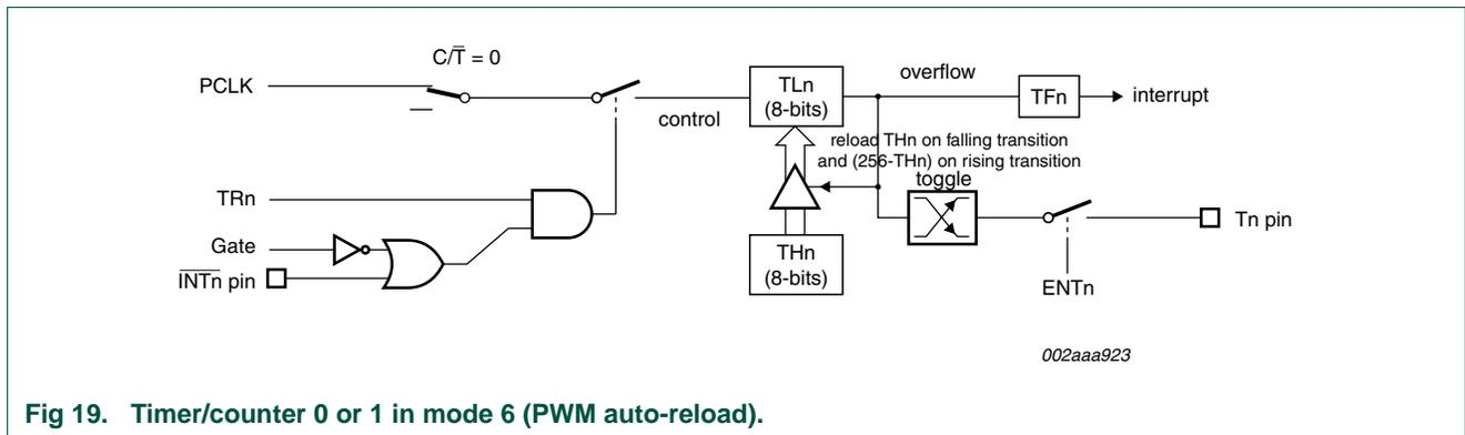
Fig 19. Timer/counter 0 or 1 in mode 6 (PWM auto-reload).
