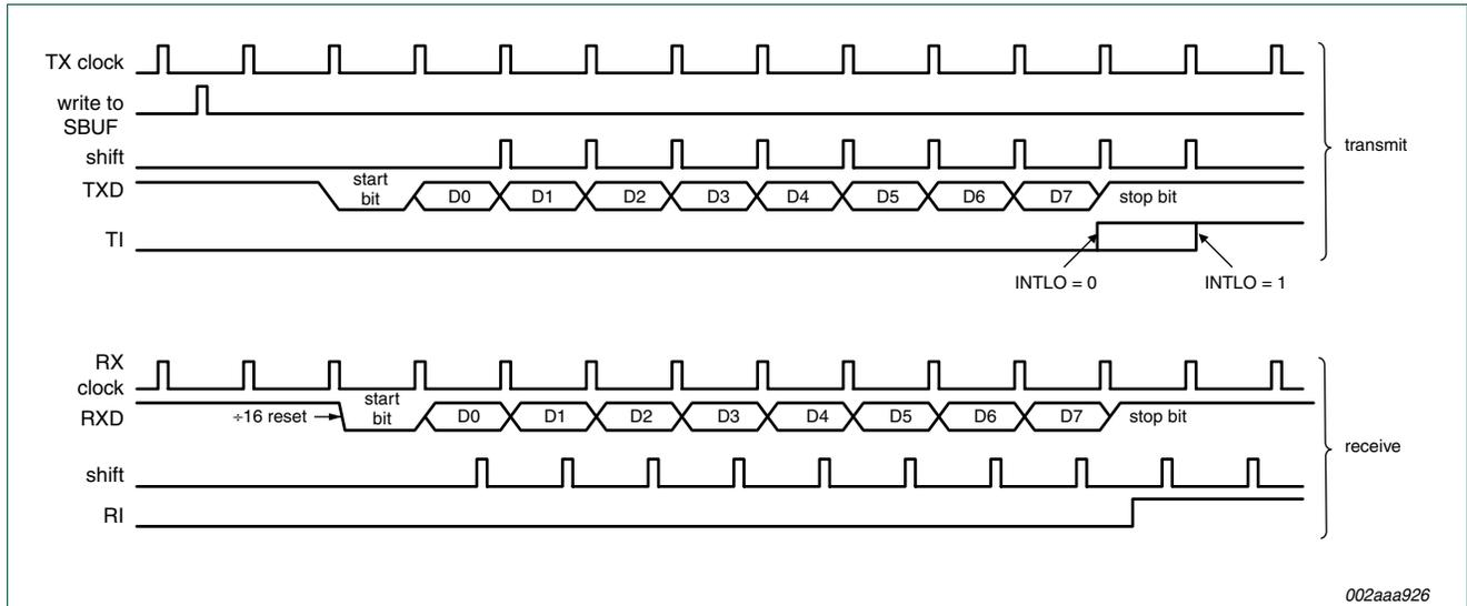
Fig 23. Serial Port Mode 1 (only single transmit buffering case is shown).
