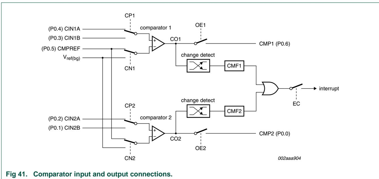
**Fig 41. Comparator input and output connections.**
