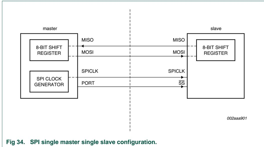
**Fig 34. SPI single master single slave configuration.**
