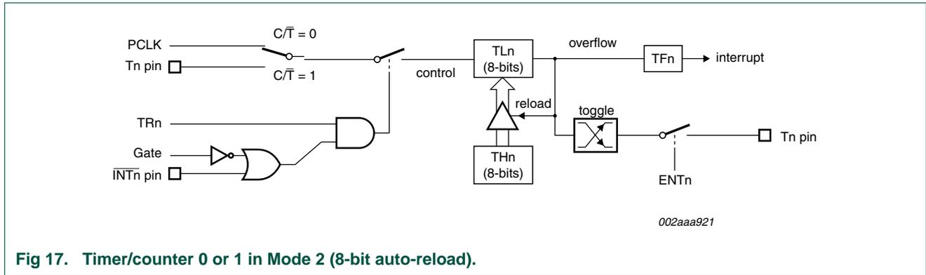
Fig 17. Timer/counter 0 or 1 in Mode 2 (8-bit auto-reload).
