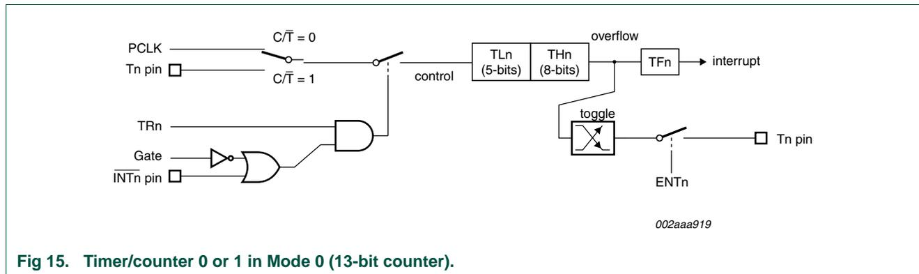
**Fig 15. Timer/counter 0 or 1 in Mode 0 (13-bit counter).**
