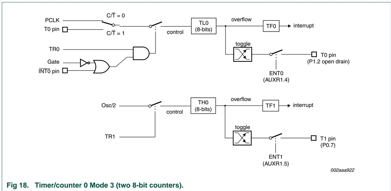
Fig 18. Timer/counter 0 Mode 3 (two 8-bit counters).
