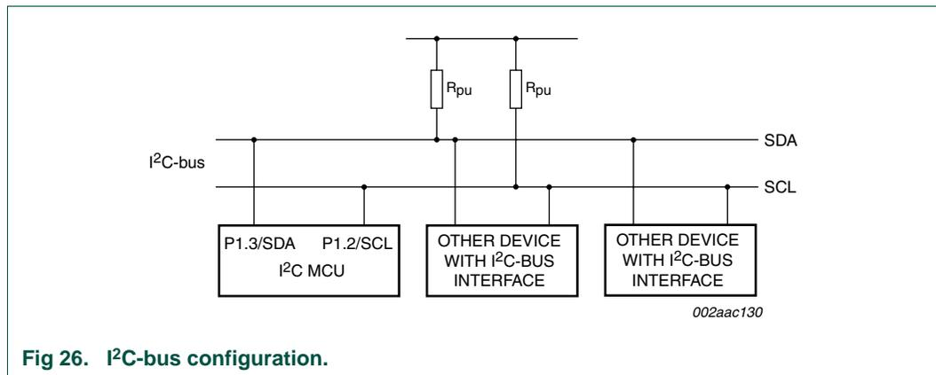
Fig 26. I<sup>2</sup>C-bus configuration.
