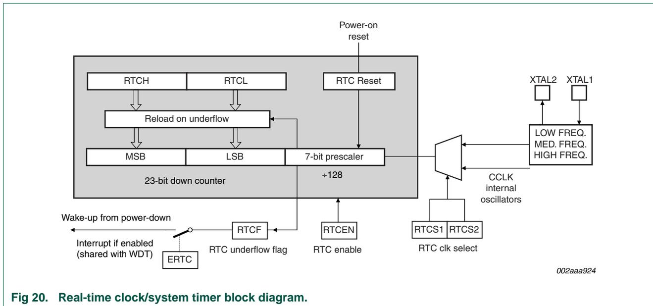
Fig 20. Real-time clock/system timer block diagram.
