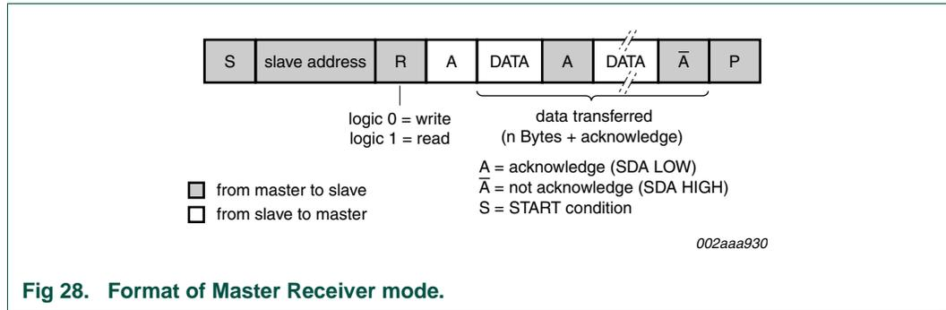
**Fig 28. Format of Master Receiver mode.**
