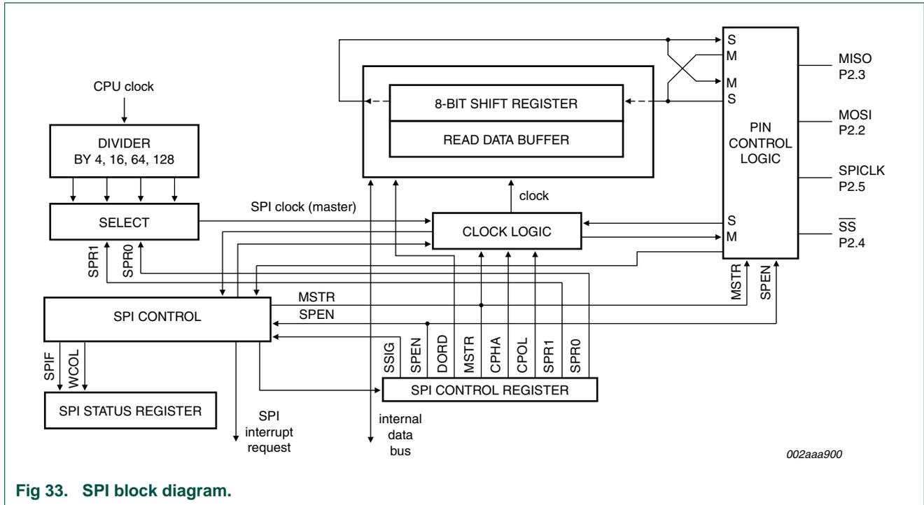
Fig 33. SPI block diagram.
