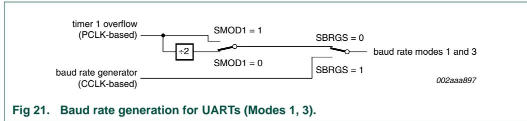
Fig 21. Baud rate generation for UARTs (Modes 1, 3).
