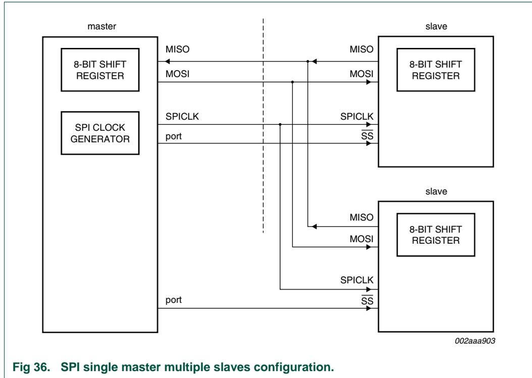
Fig 36. SPI single master multiple slaves configuration.
