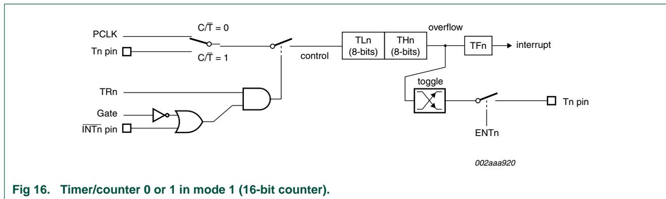
**Fig 16. Timer/counter 0 or 1 in mode 1 (16-bit counter).**
