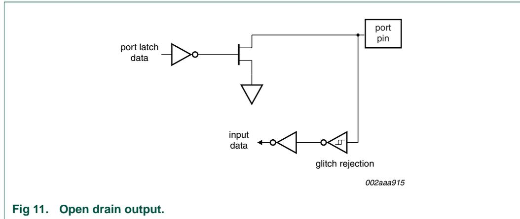
Fig 11. Open drain output.
