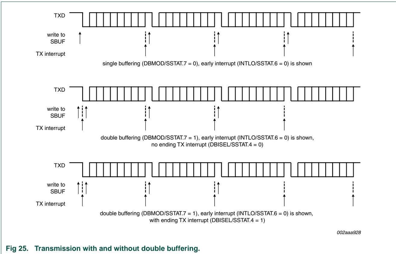
Fig 25. Transmission with and without double buffering.
