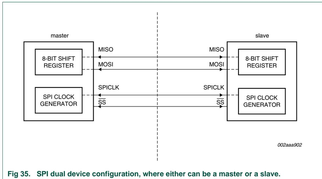
**Fig 35. SPI dual device configuration, where either can be a master or a slave.**
