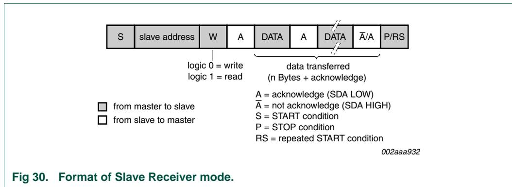
Fig 30. Format of Slave Receiver mode.
