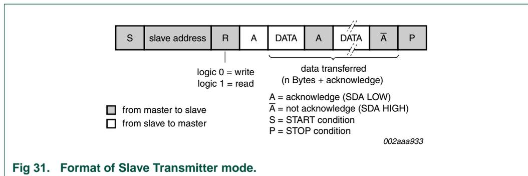
Fig 31. Format of Slave Transmitter mode.
