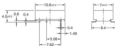
**Note:** Each value has a tolerance of  $\pm 0.3$  mm. The coplanarity of the terminals is 0.1 mm max.
