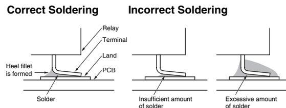
Visually check that the Relay is properly soldered.
