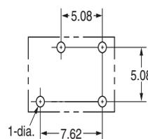
**Terminal Arrangement/ Internal Connections (Bottom View)**
