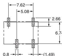
**Terminal Arrangement/ Internal Connections (Top View)**
