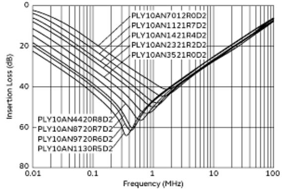
Common Mode Insertion Loss-Frequency Characteristics
