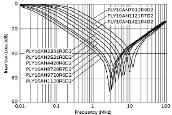
Differential Mode Insertion Loss-Frequency Characteristics
