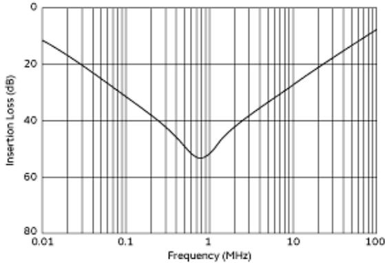
Common Mode Insertion Loss (Typ.)
