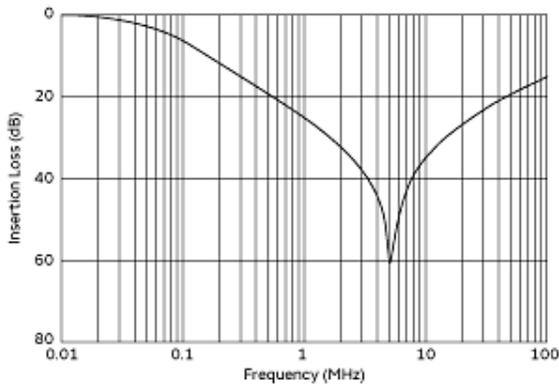
Differential Mode Insertion Loss (Typ.)
