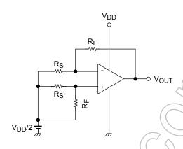
SVRR.  $V_{DD} = 1.8 \text{ V: } V_{DD} = V_{DD}1, V_{OUT} = V_{OUT}1$  $V_{DD} = 7.0 \text{ V}$ :  $V_{DD} = V_{DD}2$ ,  $V_{OUT} = V_{OUT}2$
