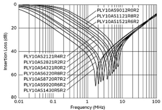
Differential Mode Insertion Loss-Frequency Characteristics
