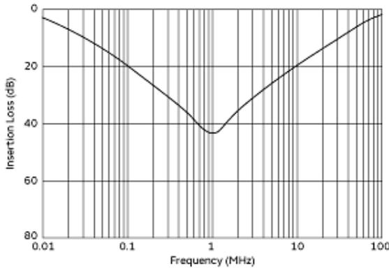
Common Mode Insertion Loss (Typ.)
