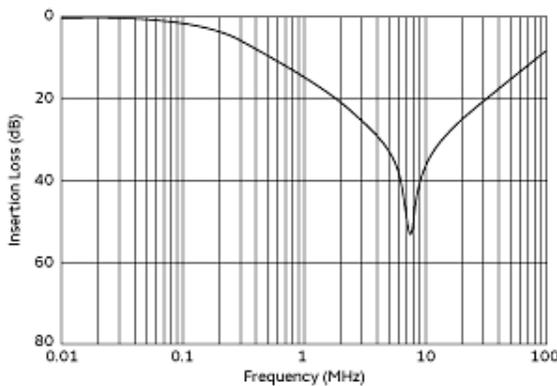
Differential Mode Insertion Loss (Typ.)
