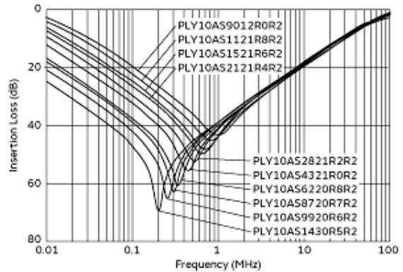
Common Mode Insertion Loss-Frequency Characteristics
