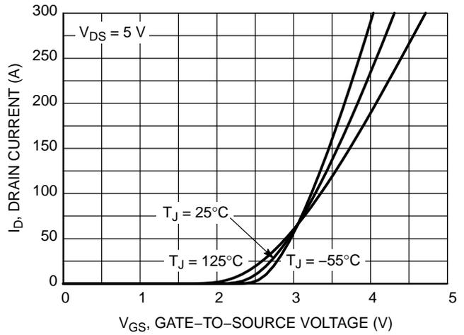
Figure 2. Transfer Characteristics
