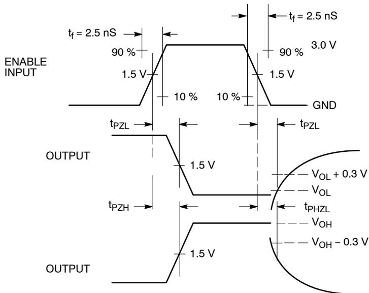
**Figure 5. Enable/Disable Delays**
