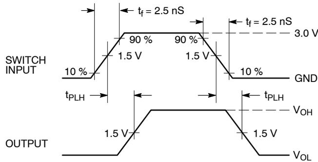
**Figure 4. Propagation Delays**
