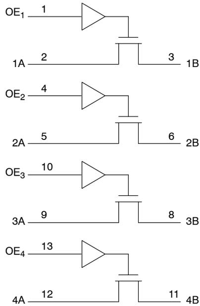
Figure 2. Logic Diagram
