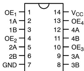
Figure 1. Pin Assignment for SOIC and TSSOP
