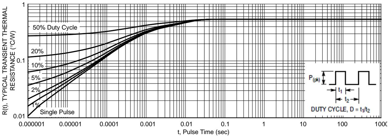
Figure 9. Typical Transient Thermal Response for NTSB20100CTG
