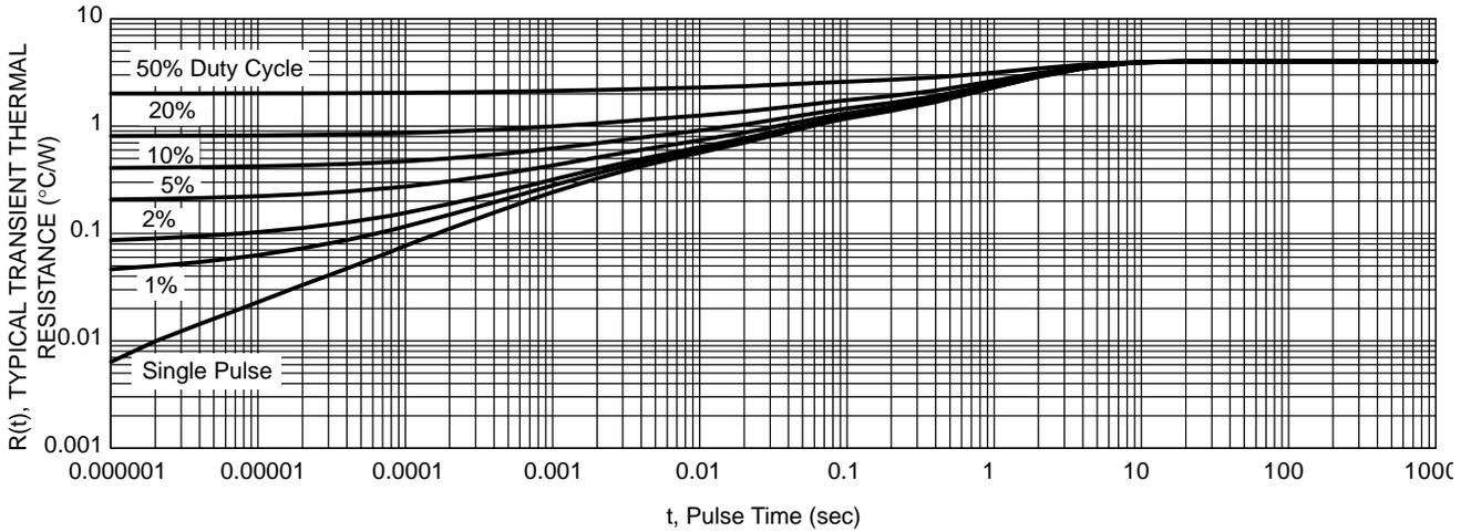
Figure 8. Typical Transient Thermal Response, Junction-to-Case for NTSJ20100CTG
