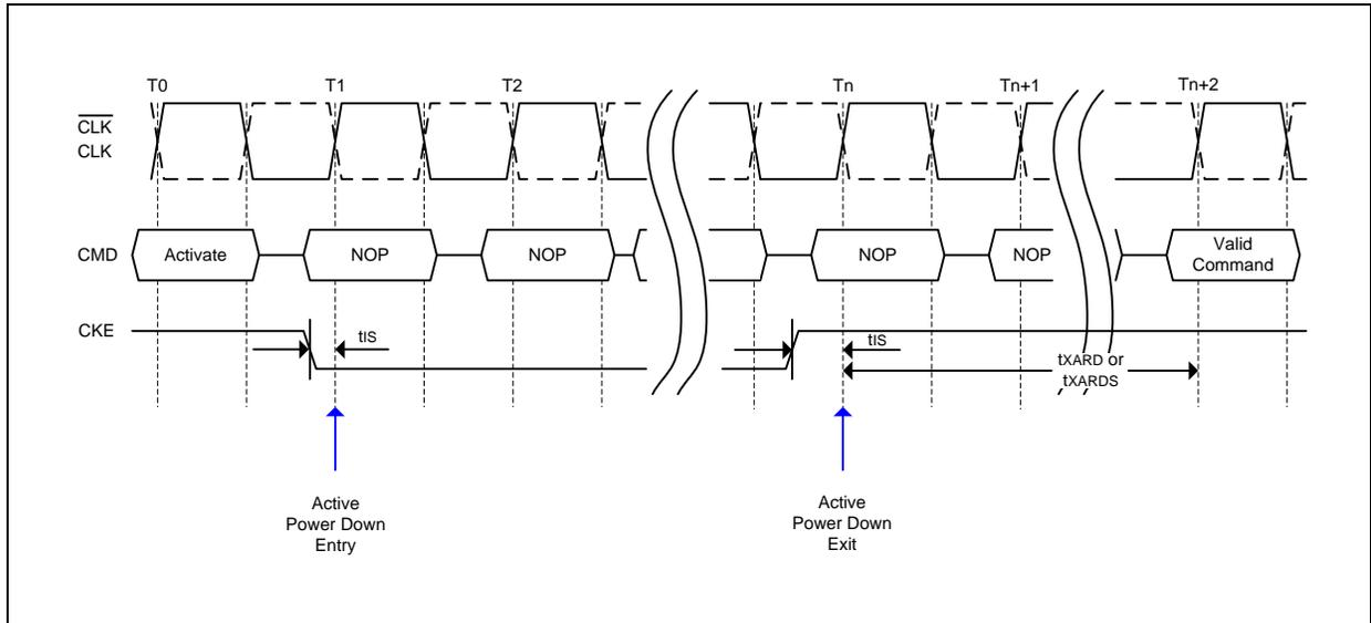
11.30 Precharged Power Down Mode Entry and Exit Timing
