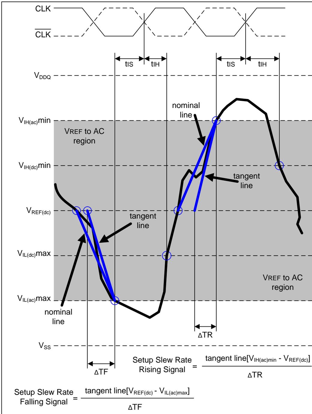
Figure 21 – Illustration of tangent line for tIS
