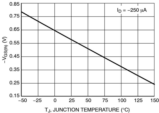
Figure 11. Threshold Voltage
