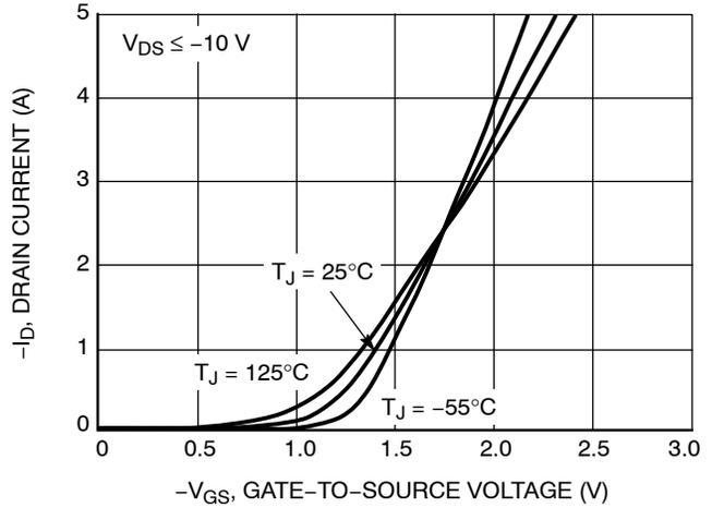
Figure 2. Transfer Characteristics
