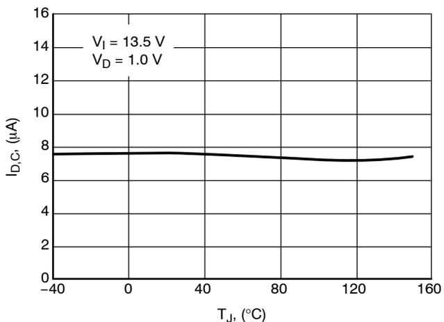
Figure 5. Charge Current  $I_{D,C}$  vs. Temperature  $T_J$
