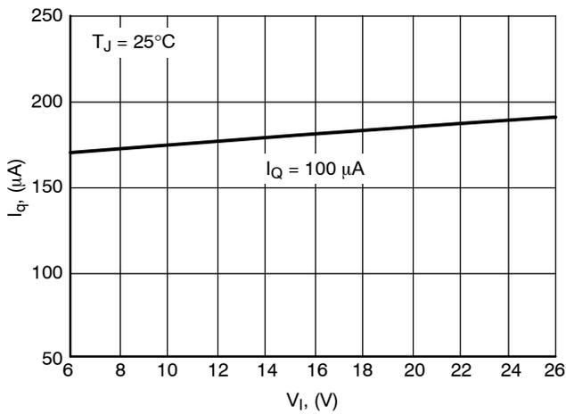
Figure 17. Quiescent Current  $I_q$  vs. Input Voltage  $V_I$
