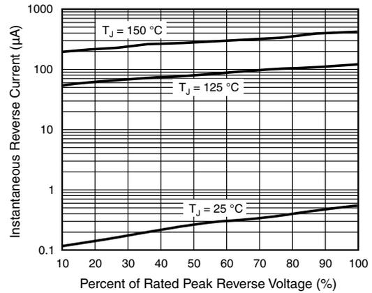
Fig. 5 - Typical Reverse Characteristics Per Diode
