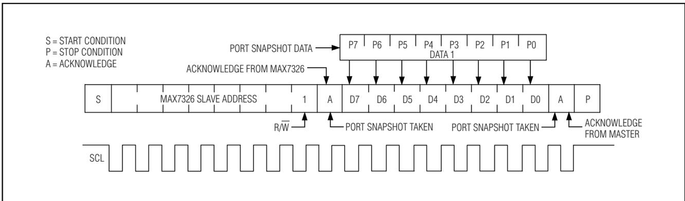
Figure 8. Reading Group B Ports of the MAX7326
