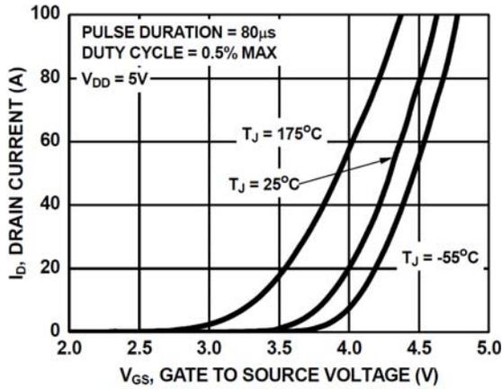
Figure 7. Transfer Characteristics
