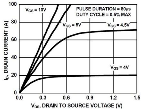
Figure 8. Saturation Characteristics
