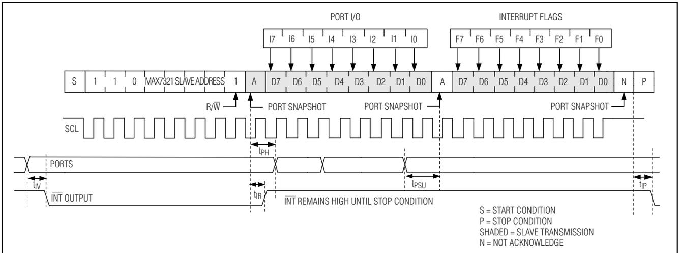
Figure 7. Reading the MAX7321 (2 Data Bytes)
