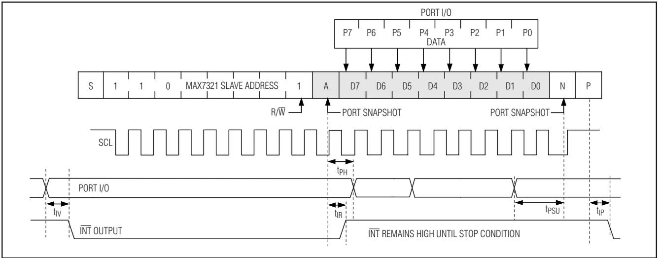
Figure 6. Reading the MAX7321 (1 Data Byte)
