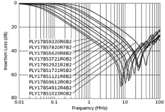
Differential Mode Insertion Loss-Frequency Characteristics
