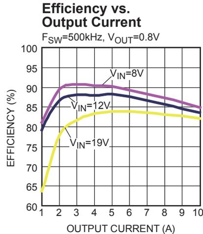
Figure 21 — Efficiency Curve
