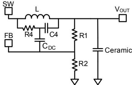
**Figure 9—Simplified Ceramic Capacitor Circuit with DC-Blocking Capacitor**
