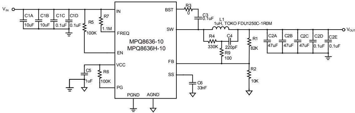
**Figure 50 — Typical Application Circuit with Low ESR Ceramic Capacitor**
