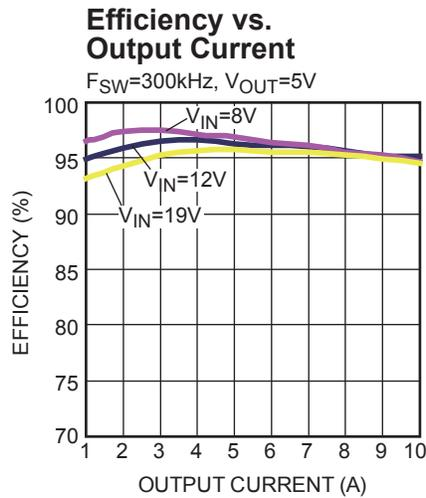
**Figure 47 — Efficiency Curve**
