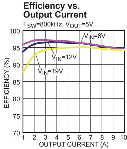
Figure 17 — Efficiency Curve
