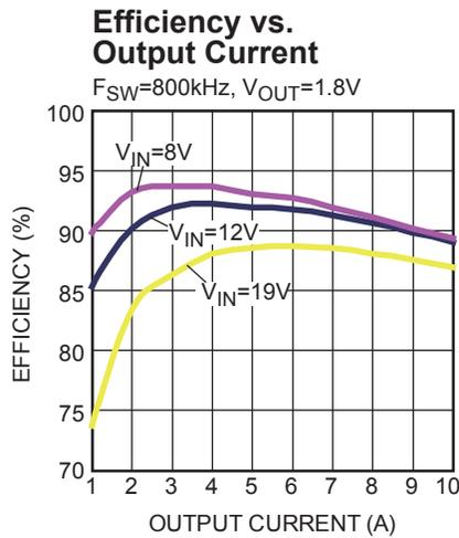
Figure 39 — Efficiency Curve
