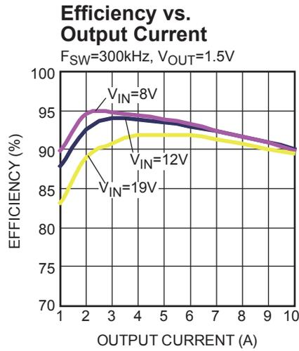
**Figure 29 — Efficiency Curve**
