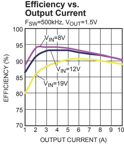
**Figure 31 — Efficiency Curve**
