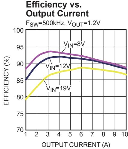
Figure 25 — Efficiency Curve
