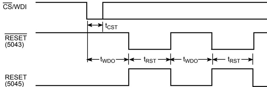
**RESET/RESET Output Timing**
