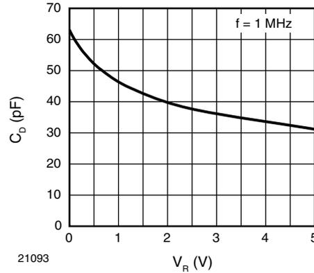
Fig. 6 - Typical Capacitance  $C_D$  vs. Reverse Voltage  $V_R$
