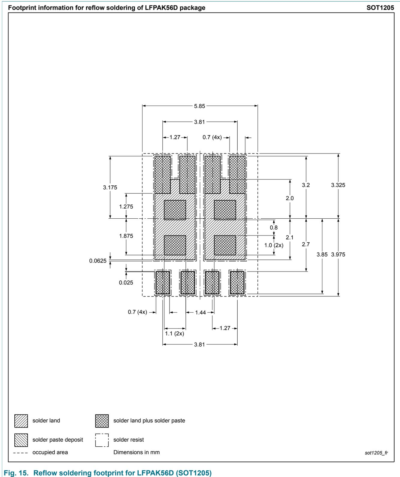
Fig. 15. Reflow soldering footprint for LFPAK56D (SOT1205)
