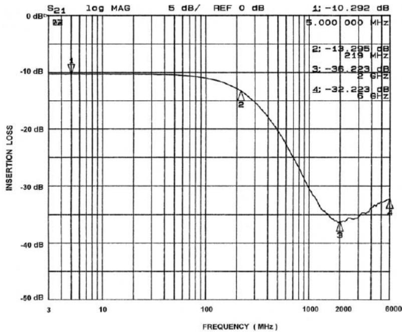
Figure 6. Channel 2 EMI Filter Performance (CM1407-08)
