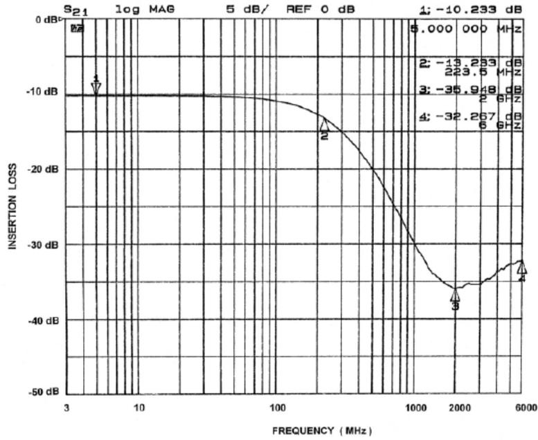
Figure 7. Channel 3 EMI Filter Performance (CM1407-08)
