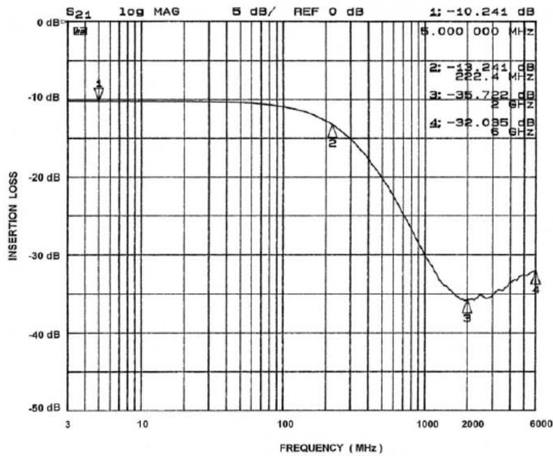
Figure 10. Channel 6 EMI Filter Performance (CM1407-08)
