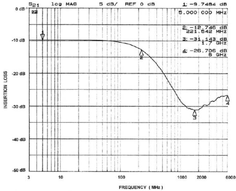
Figure 1. Channel 1 EMI Filter Performance (CM1407-04)
