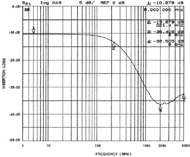
Figure 11. Channel 7 EMI Filter Performance (CM1407-08)
