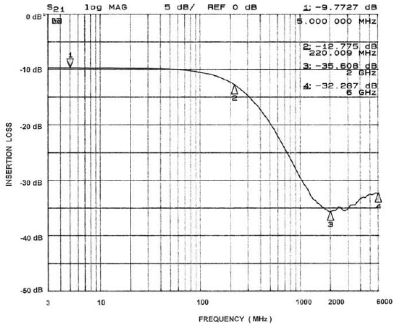
Figure 2. Channel 2 EMI Filter Performance (CM1407-04)
