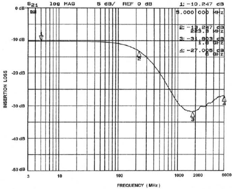
Figure 5. Channel 1 EMI Filter Performance (CM1407-08)
