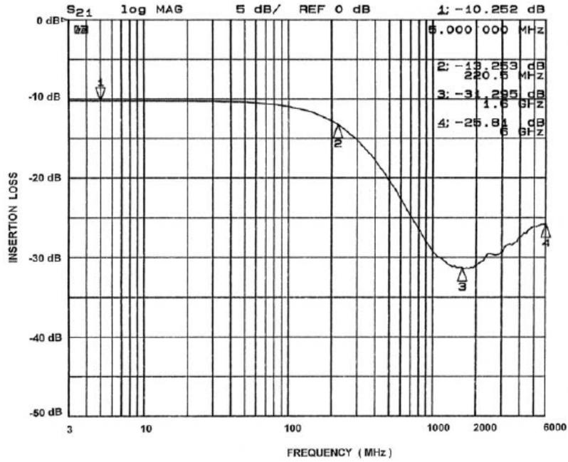
Figure 9. Channel 5 EMI Filter Performance (CM1407-08)
