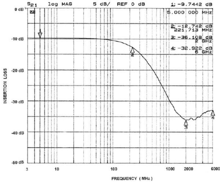
Figure 3. Channel 3 EMI Filter Performance (CM1407-04)
