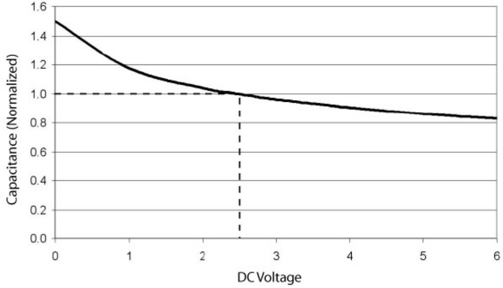
**Figure 13. Filter Capacitance vs. Input Voltage over Temperature
