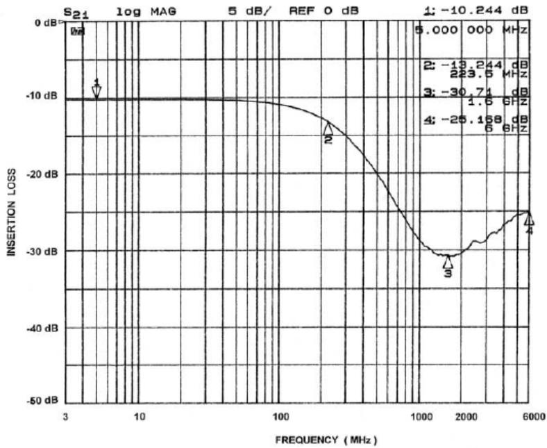
Figure 8. Channel 4 EMI Filter Performance (CM1407-08)
