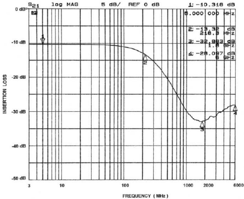
Figure 12. Channel 8 EMI Filter Performance (CM1407-08)
