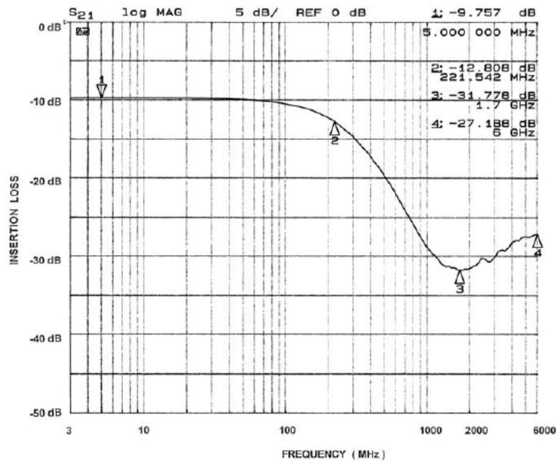
Figure 4. Channel 4 EMI Filter Performance (CM1407-04)
