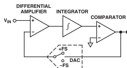
Figure 5. Basic Charge-Balancing ADC
