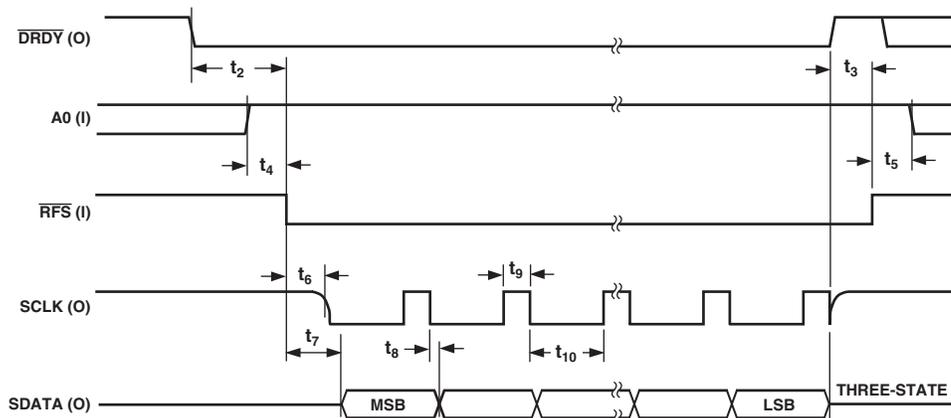
Figure 10. Self-Clocking Mode, Output Data Read Operation
