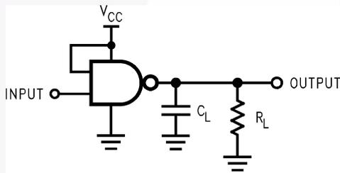
C<sub>L</sub> includes load and stray capacitance
