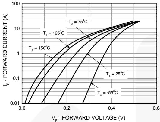
**Figure 3. Typical Forward Characteristics**
