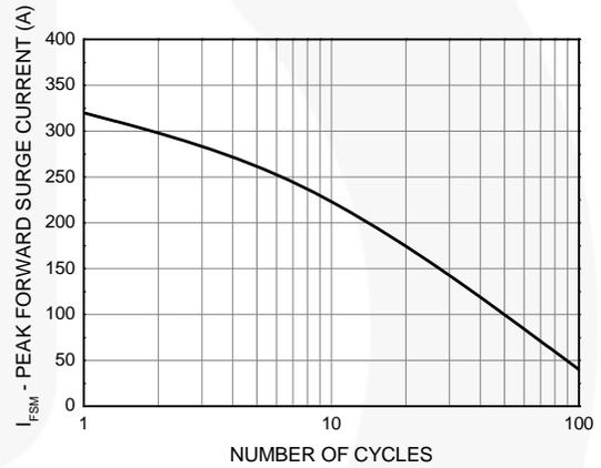
**Figure 6. Maximum Non-Repetitive Peak Forward Surge Current**
