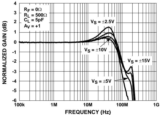
FIGURE 16. GAIN vs FREQUENCY FOR VARIOUS SUPPLY SETTINGS
