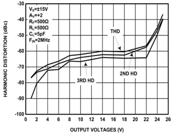
FIGURE 20. HARMONIC DISTORTION vs OUTPUT VOLTAGE ( $A_V = +2$ )
