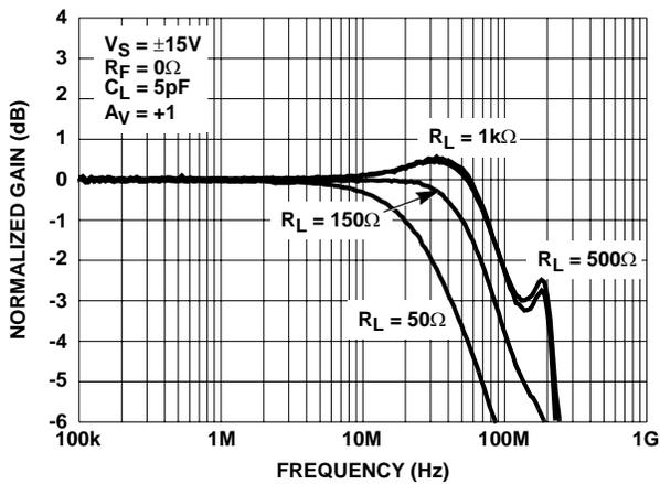
FIGURE 9. GAIN vs FREQUENCY FOR VARIOUS  $R_{LOAD}$  ( $A_V = +1$ )
