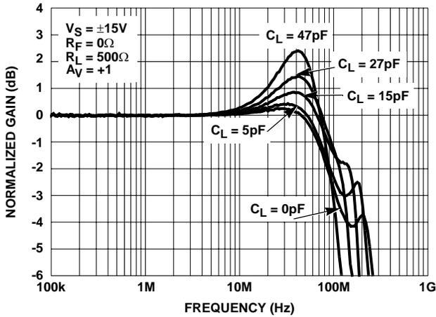
FIGURE 11. GAIN vs FREQUENCY FOR VARIOUS  $C_{LOAD}$  ( $A_V = +1$ )
