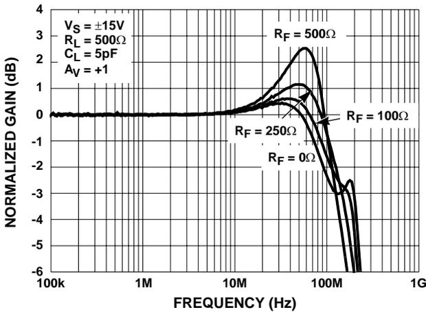
FIGURE 13. GAIN vs FREQUENCY FOR VARIOUS  $R_{FEEDBACK}$  ( $A_V = +1$ )
