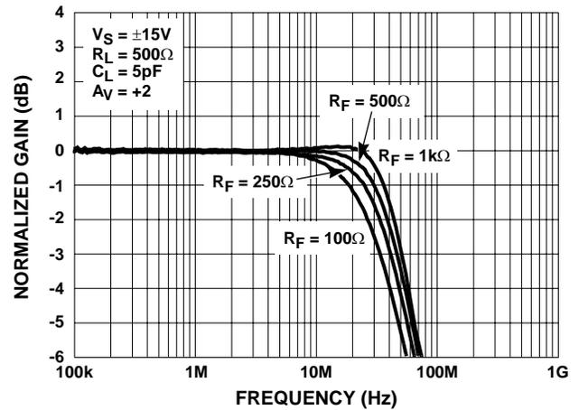
FIGURE 14. GAIN vs FREQUENCY FOR VARIOUS  $R_{FEEDBACK}$  ( $A_V = +2$ )
