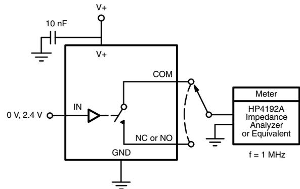
Fig. 5 - Channel off/on Capacitance
