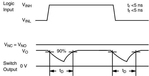
Fig. 2 - Break-Before-Make Interval
