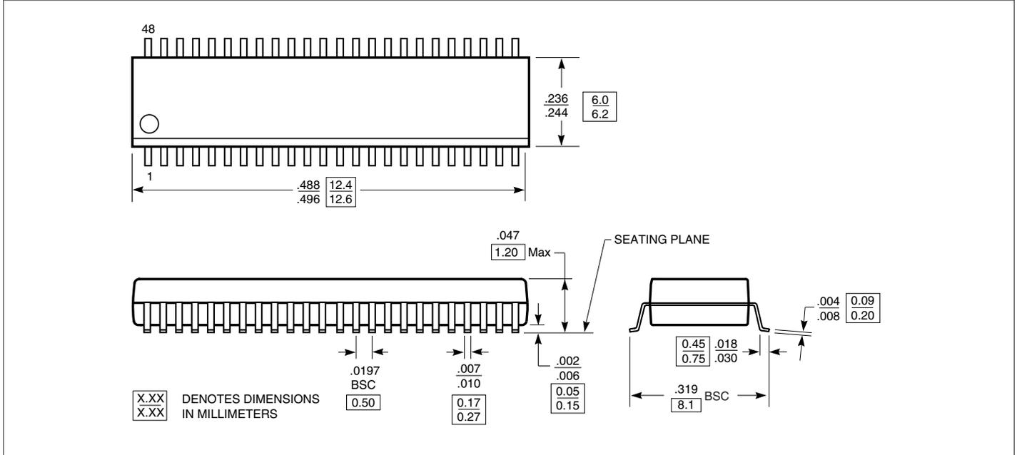
**Packaging Mechanical: 48-pin SSOP (V)**
